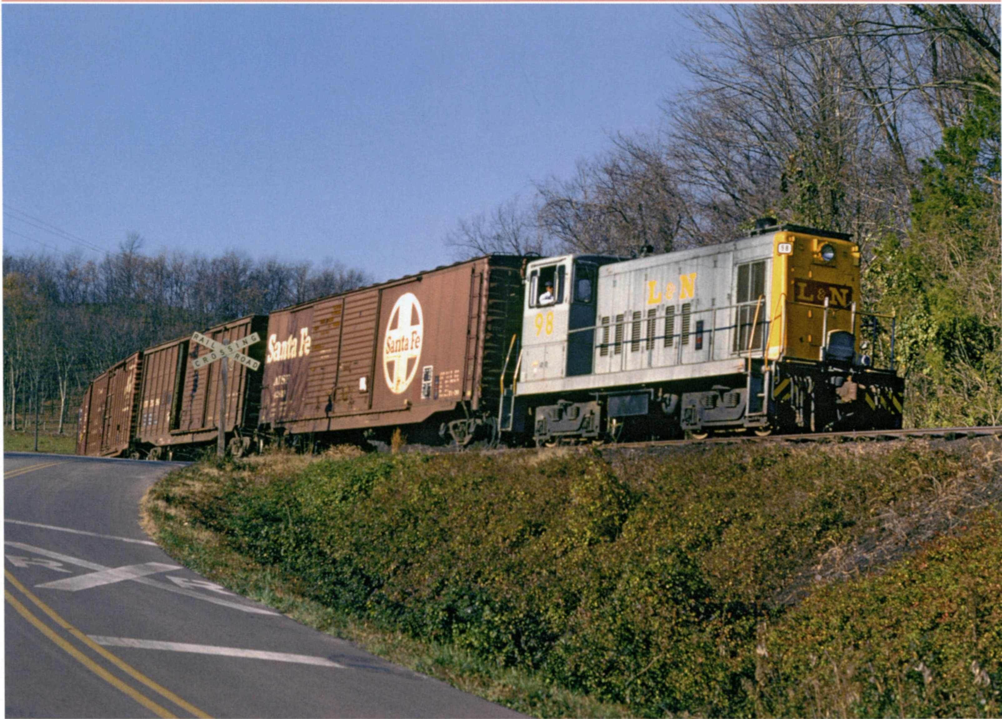
GE 70-tonner number 98 is about two miles west of the end of the branch at Hartsville, TN, on November 19, 1977, as it crosses a highway at Stovall Gap. One of two on the roster, the 98 was repowered at South Louisville in 1966 with an 800 HP Alco 6-251B diesel prime mover (200 more horsepower than the GE prime mover). The rebuild required raising the hood considerably. It was sold to Tropicana in 1980 to switch orange juice. —David M. Johnston photo
