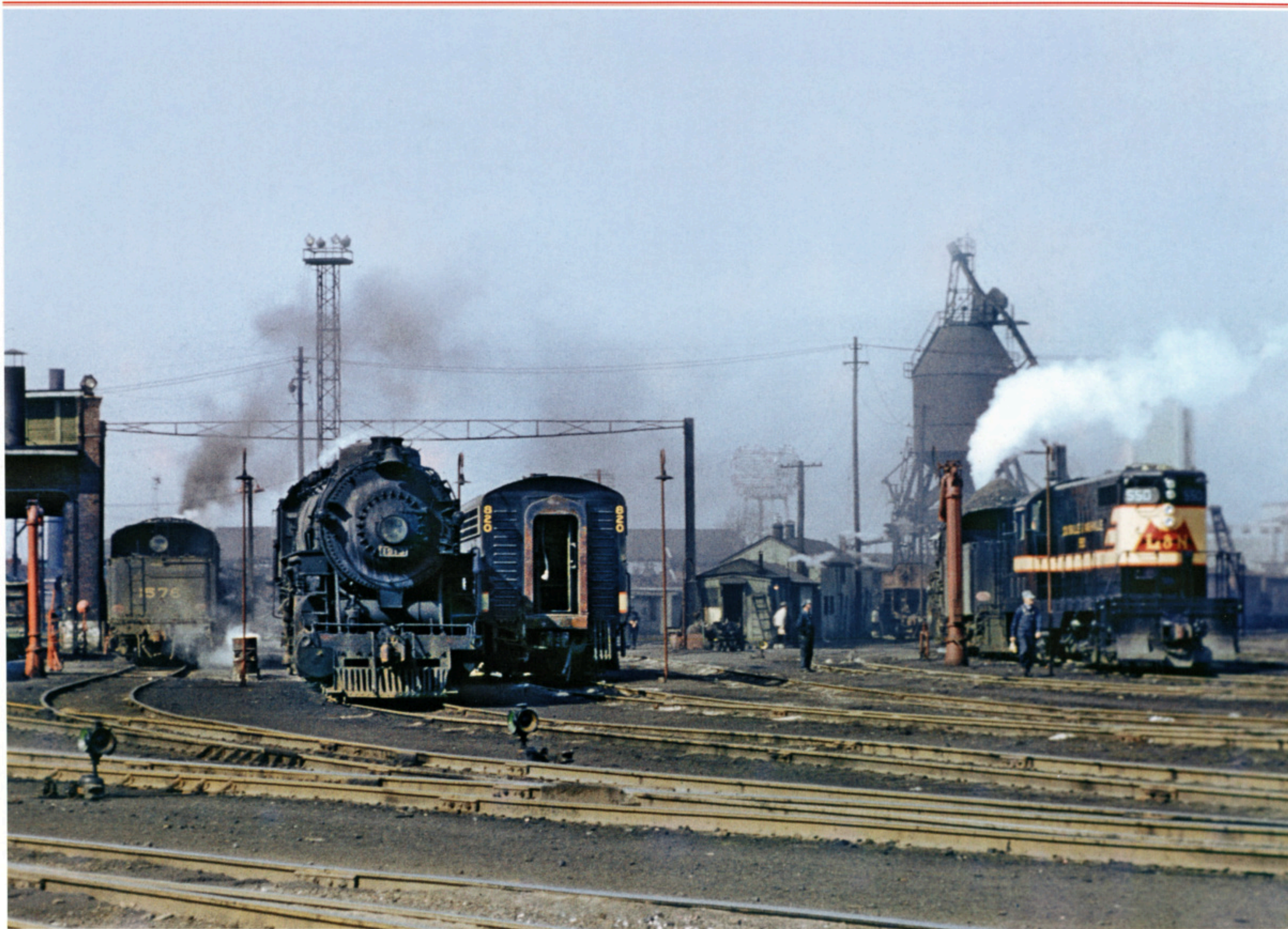
In a scene from April 1951, the steam to diesel transition period on the L&N is in full swing at South Louisville. Left to right is the tender of J-3 number 1576, J-4A number 1913, F7A number 820, and brand-new GP7 number 550. Another steam locomotive is behind the 550, but the number isn't visible. Notice the GP7 does not have MU capability. That feature will come later. — Jack Fravert photo
