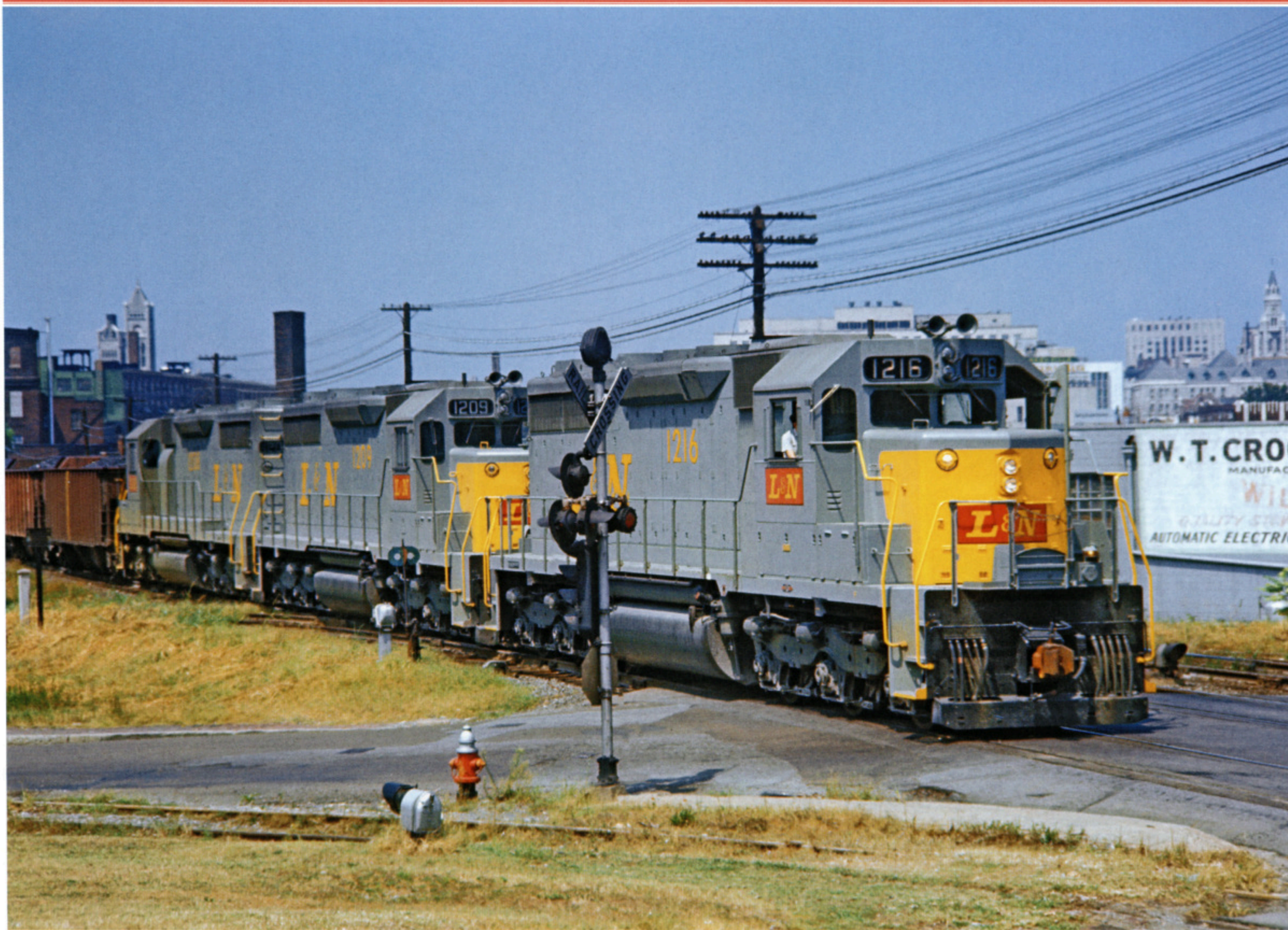
Three brand-new EMD SD35s are coming through downtown Nashville pulling a unit coal train off the Henderson Subdivision on August 29, 1965. The three shiny SDs will come off at Kayne Avenue to be replaced by five four-motor units. The coal is destined for Florence, AL, on the NF&S, and six-motor power is banned there. — Theo E. Sommerkamp photo
