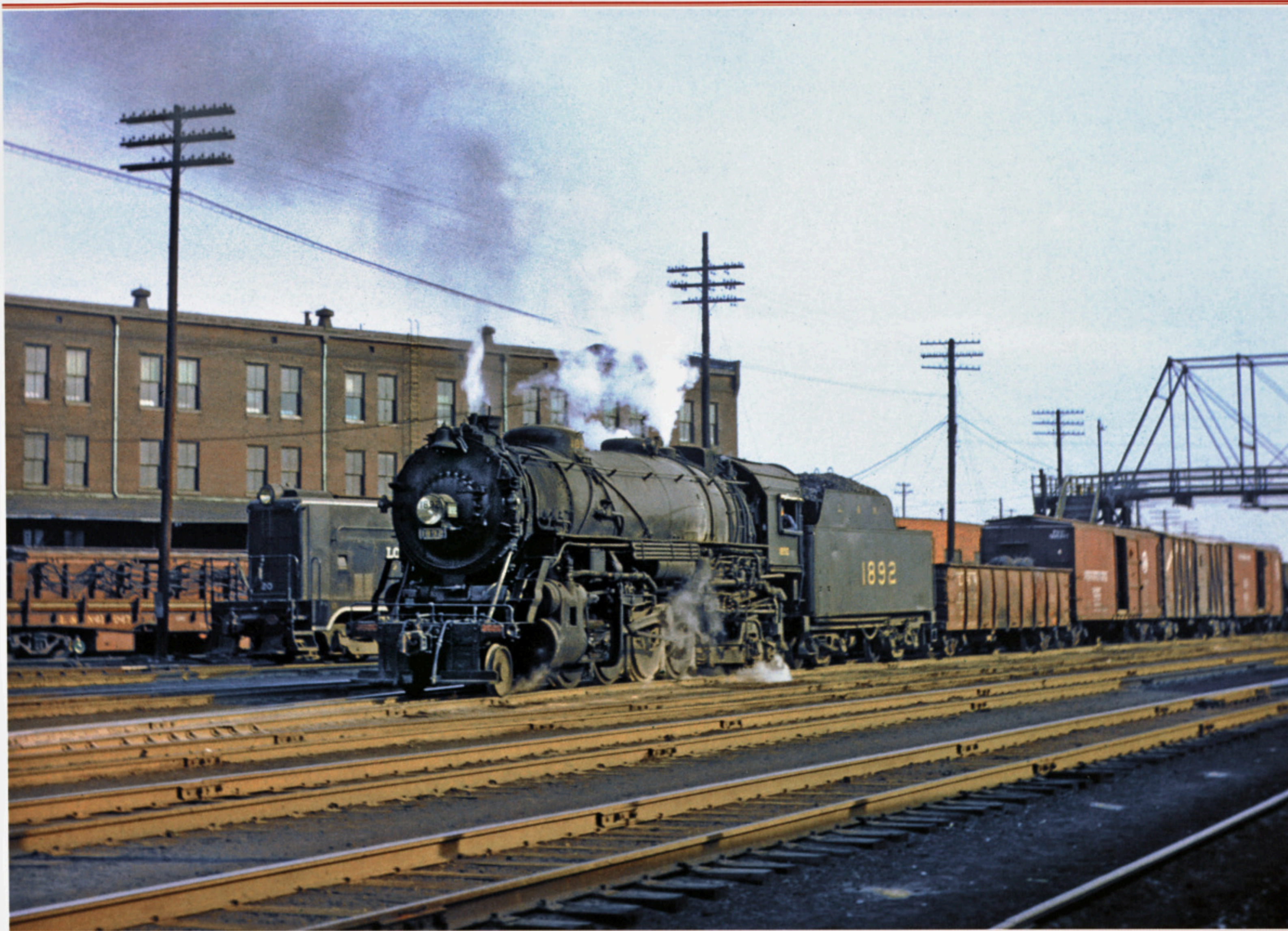
The Short Line engineer on J-4A 1892 has engaged the trailing truck booster to help get his heavy freight underway for DeCoursey in this early 1950s view at South Louisville. The 29 engines of this class were built by Baldwin in 1929, and came equipped with Delta trailing trucks. The L&N added the Franklin boosters, which added 12,075 additional pounds of starting tractive effort. The 165 engines in the J-4 and J-4A classes were all based on the USRA heavy Mikado design, but only the "sport model" J-4As had boosters. — Jack Fravert photo
