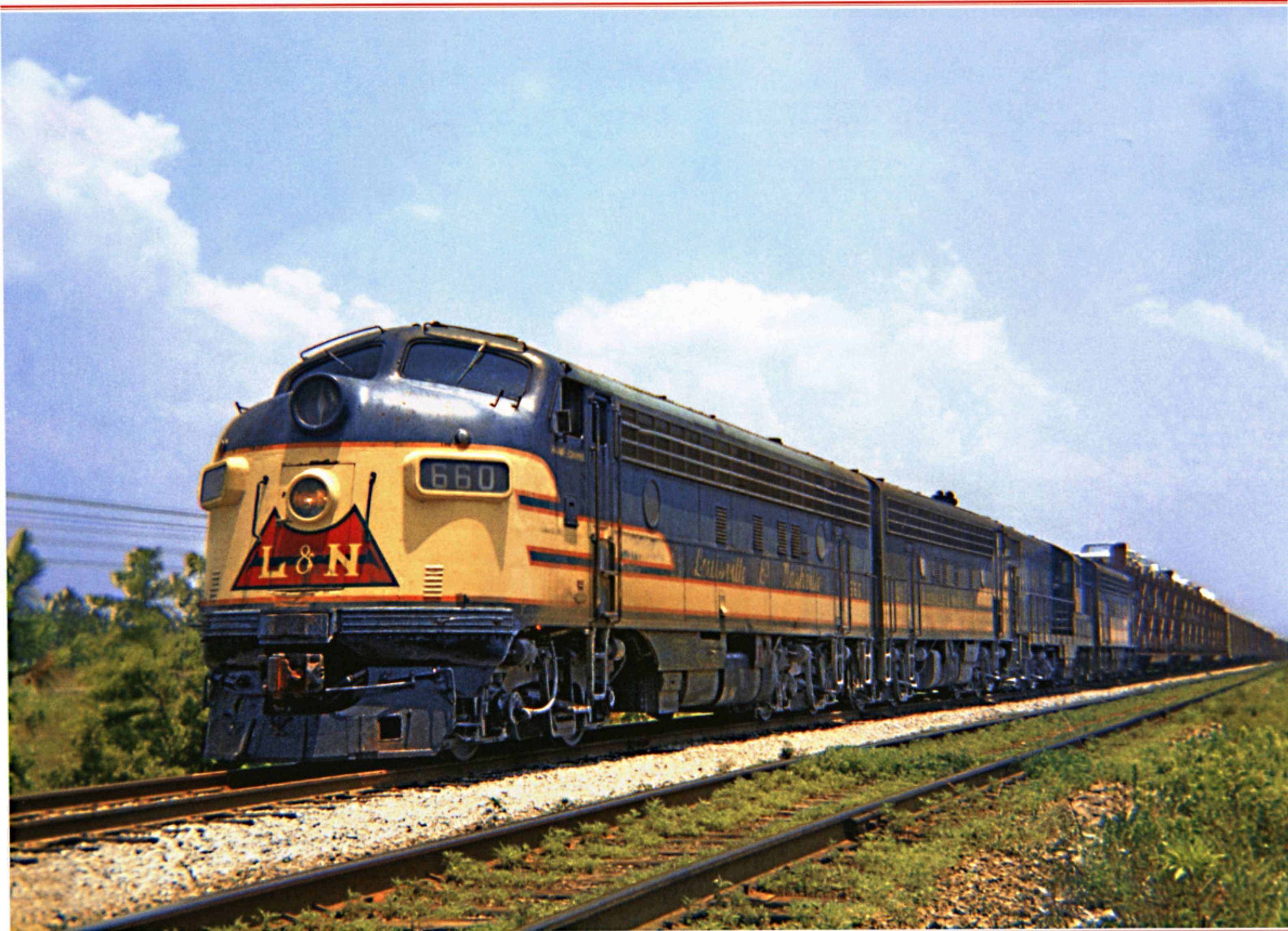
L&N Southbound train 83 is shown in this June 30, 1961 portrait at Orange Grove, Mississippi. Locomotives include 660-909-400 and 917 (FP7-F7A-GP7-F7A). Notice the loaded open tri-level auto racks first out behind the power. Sadly, en route vandalism and theft eventually required the totally enclosed rack cars that handle this traffic today. The passing siding at Orange Grove is a few miles north of Pascagoula, where the photographer worked for many years during his days as an operator. — Jerry G. Lachaussee photo
