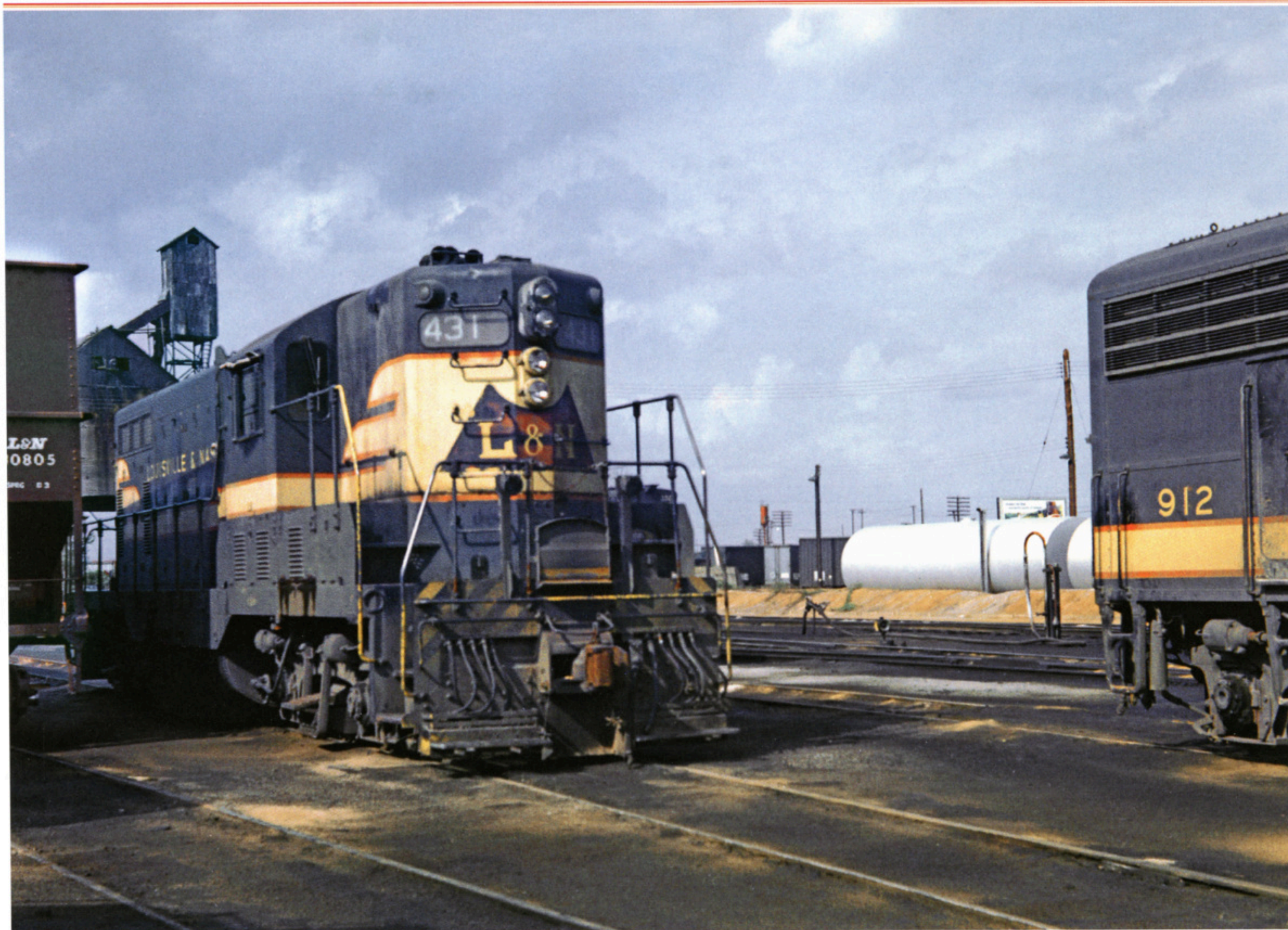
L&N At Montgomery, Alabama on April 7, 1964, GP7 number 431 and F7 number 912 await calls to duty. The old steam-era coaling station was still standing, since it was still being used for locomotive sand. The hopper on the left with the extended top is a 70-ton wood chip car. This is one of many hoppers initially used primarily to carry coal that were converted at South Louisville in the early 1960s. —Jerry G. Lachaussee photo
