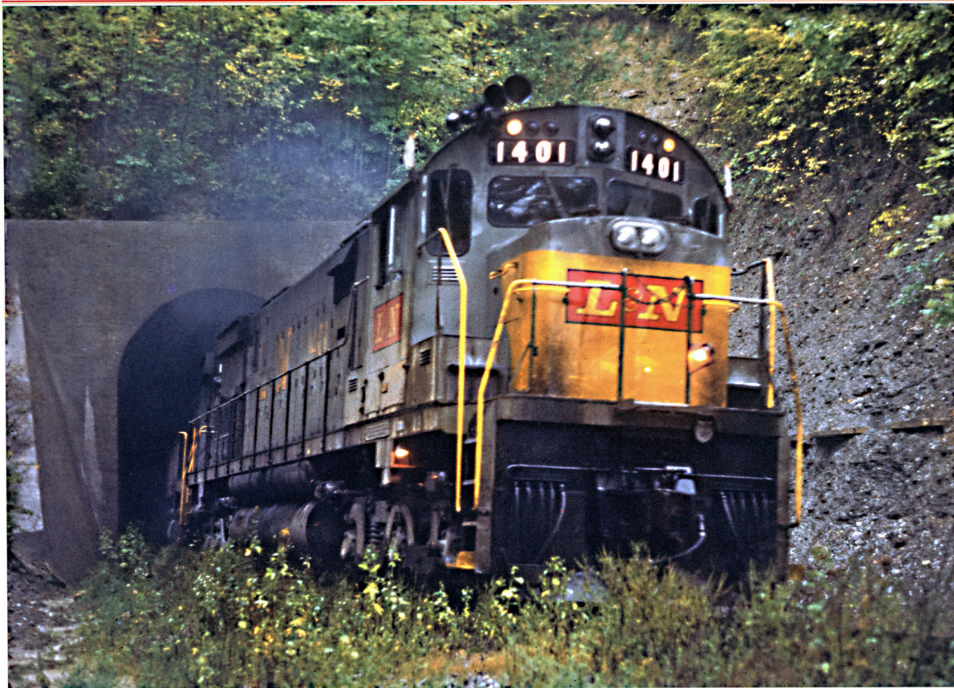
In a haze of exhaust smoke, a southbound CV Division Lynch Turn blows out Gap Ridge Tunnel near Rhea, Kentucky, on the Poor Fork Branch. The white flags and illuminated classification lights denote this as an un-scheduled or "extra" run in timetable-train order territory. This 1965 shot epitomizes the look and feel of the L&N's coalfield lines at that time. The big Alco C-628s like 1401 were always filthy from such service. Obviously the weed spray train hasn't been this way in a while. —Jim Boyd photo
