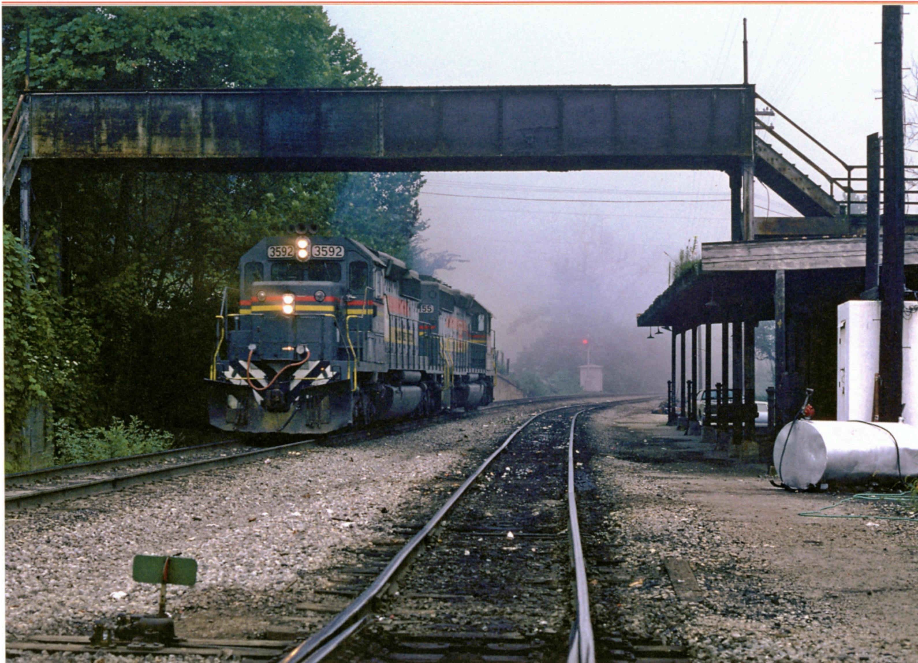
On the foggy morning of August 14, 1982, the Elkatawa Hill helper crew eases down the main line at Jackson, Kentucky to position for the shove of the next northbound coal train. All tonnage trains got a rear-end push up the hill to Chenowee Tunnel at Yeadon. Normal power for the helper was two six-motor units or three four-motor units. —Mike Leach photo, David P. Oroszi collection
