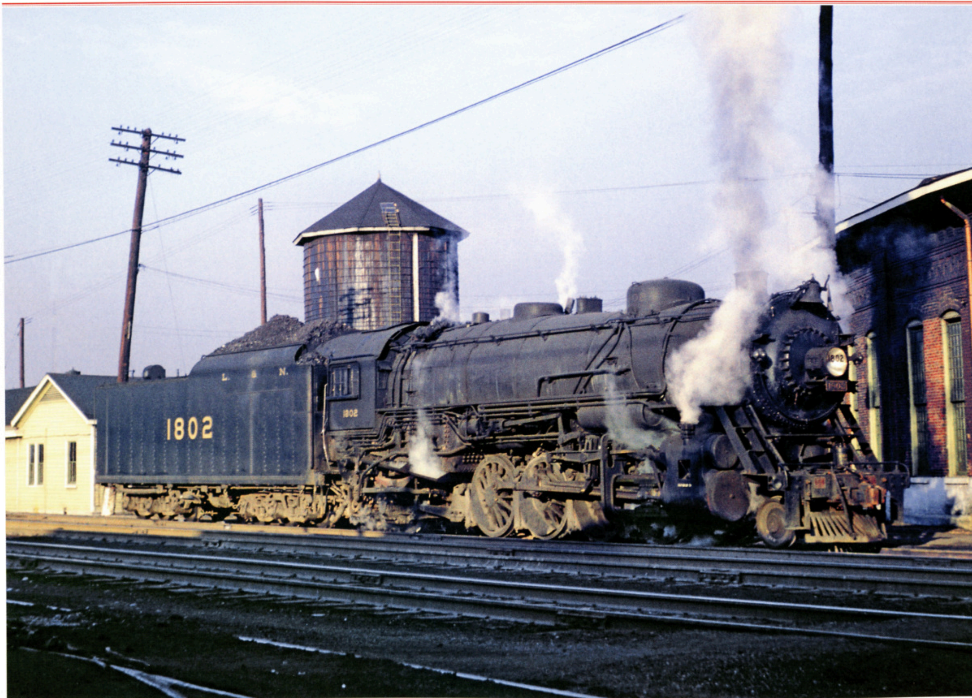
In the transition years from steam to diesel, the L&N sought to extend the range of some of its main line steam locomotives by adding larger capacity tenders and/or auxiliary water tenders, all designed to reduce the number of stops for coal and/or water. After World War II, several J-4 class Mikes acquired ex-Pere Marquette tenders from the C&O, including the 1802, shown behind the South Louisville roundhouse in 1951. Her coal bunker is full, so she's likely called to take a freight train south. — Jack Fravert photo
