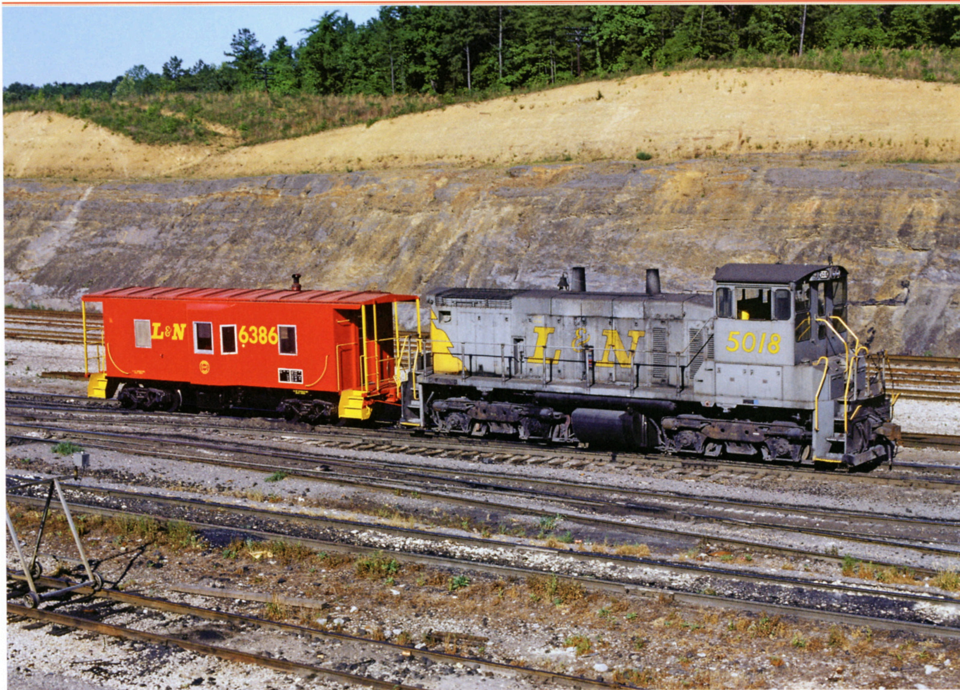
L&N At Birmingham's Boyles Yard in April 1976, SW1500 number 5018 is rolling by with bright red cab number 6386 in tow. The switcher is one of 30 units of that particular EMD model—1500 horsepower. The caboose was part of a series constructed at South Louisville in 1971—the last new cabooses to be built by the L&N. This particular cab was originally numbered 1386, but it was later renumbered. Although it was painted red when built, it has obviously just received a fresh coat. —David E. Harris photo
