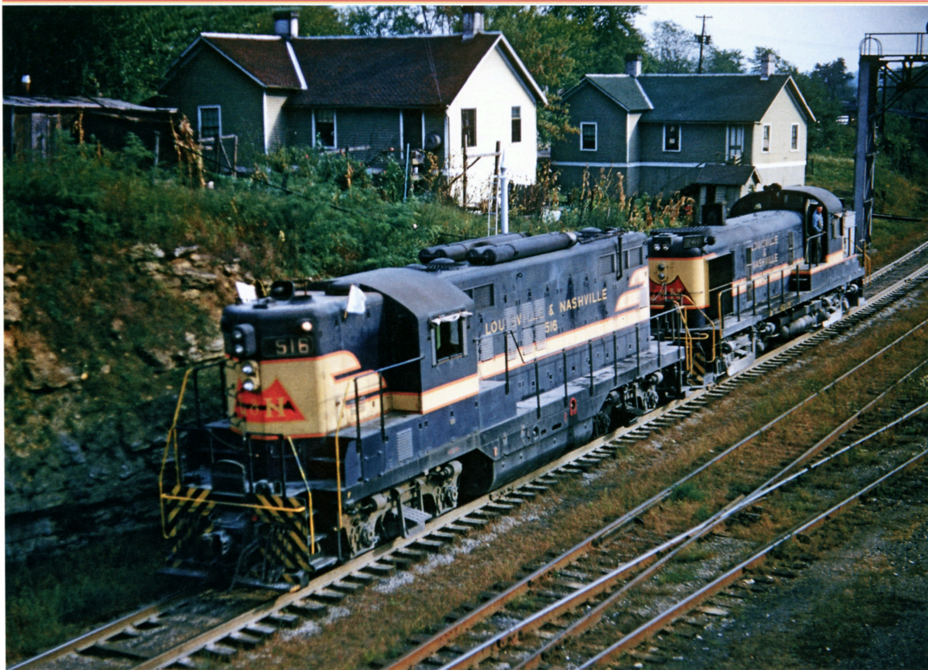
On October 2, 1957, a northbound Eastern Kentucky Division extra has cut off its train to do some switching at Patio, the busy junction and interlocking tower just south of the passenger station in Winchester, Kentucky. Both GP9 516 and RS-3 240 are dual-service units, with a steam generator and signal lines for passenger service. The four air reservoirs are mounted on top of the 516 to leave room for 1,100 gallons of water storage below, adjacent to the fuel tank. The Alco's water storage tank is above the fuel tank. —James EuDaly photo
