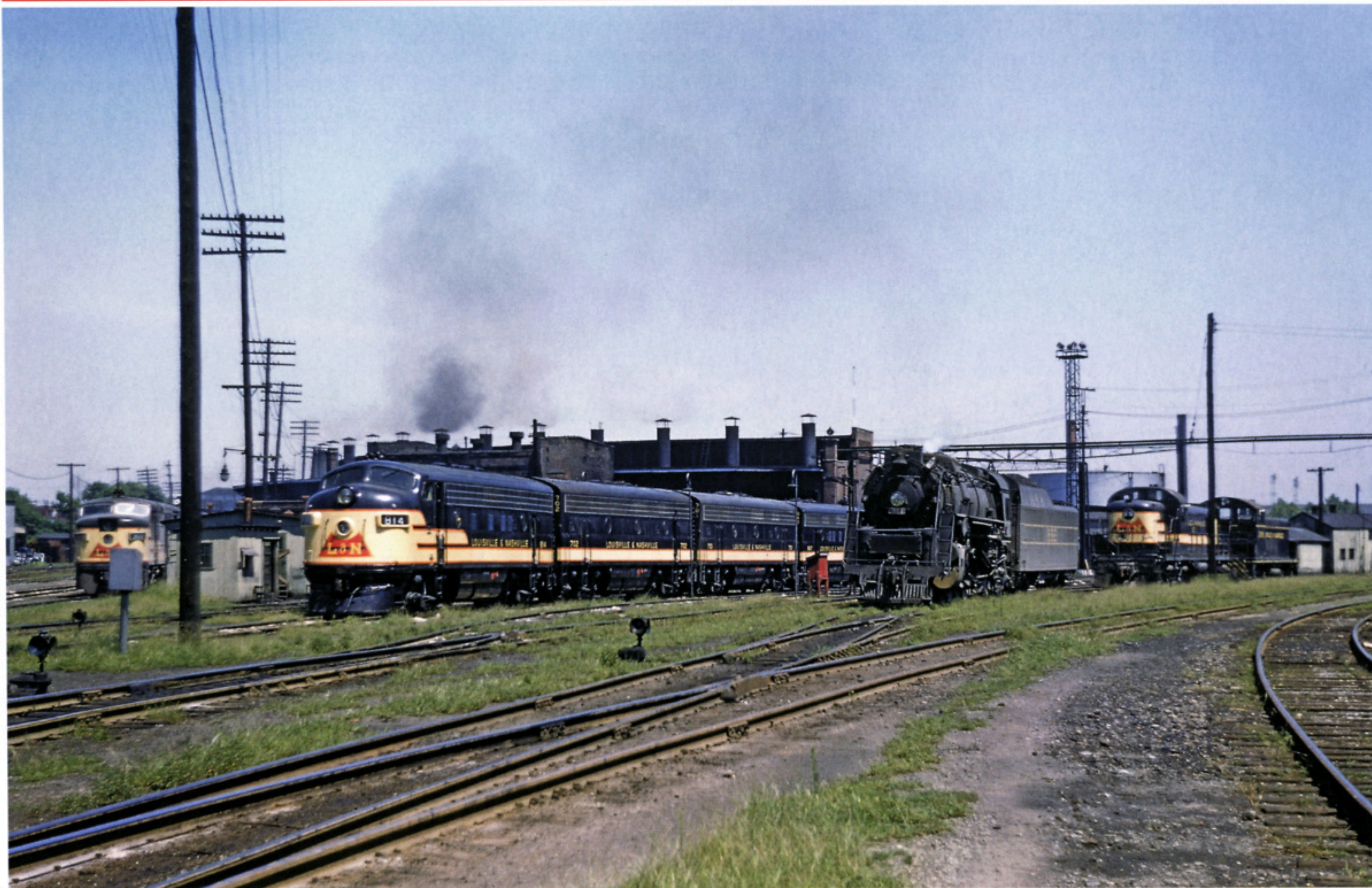
L&N Diesels are clearly dominating the motive power assignments at South Louisville in this scene from the early '50s. An Alco FA-2 cab unit is on the far left—probably assigned to Lebanon Branch trains to Corbin. The A-B-B-A F7 set would be working the Main Stem. M-1 number 1982 most likely worked its way to South Louisville from DeCoursey, while the RS-3 is power for a local freight. The SW7 is one of many yard engines assigned to the Louisville terminal area. But—smoke rising from one of the smoke jacks in the roundhouse tells us at least one other steam locomotive is fired up and ready for service. — Jack Fravert photo
