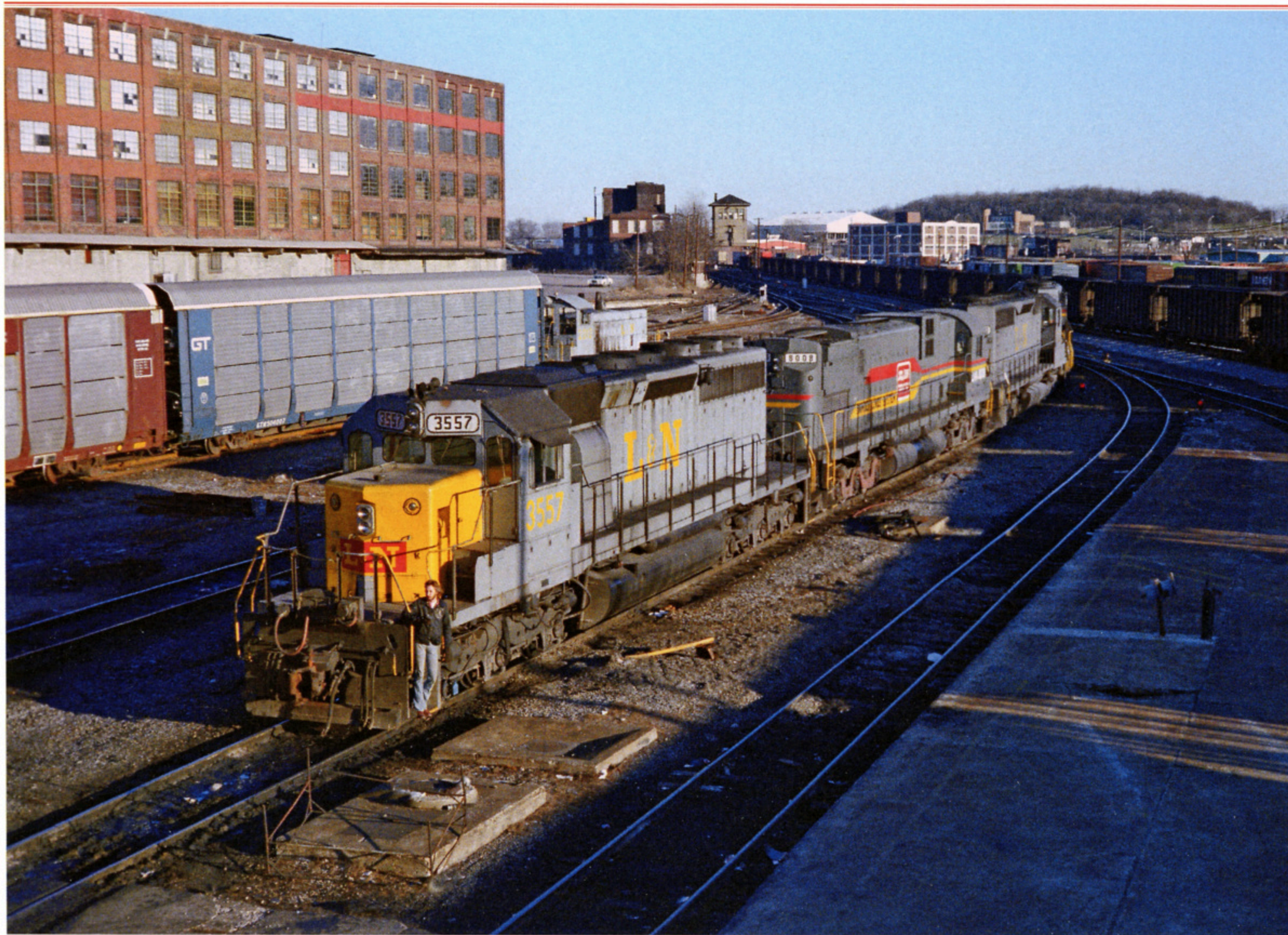
The power for a Stilesboro unit coal train backs into Track 10 at Nashville Union Station in early 1979. South End tower is in the background. This tower, as well as Church Street tower on the north side of the passenger terminal, were rather unique in being constructed atop structures straddling the tracks. The three EMD SD40-2s are assisted by a single Alco — C-630 number 8008, a former SCL (earlier, ACL) unit added to the roster in May 1977. — Doug Roberts photo
