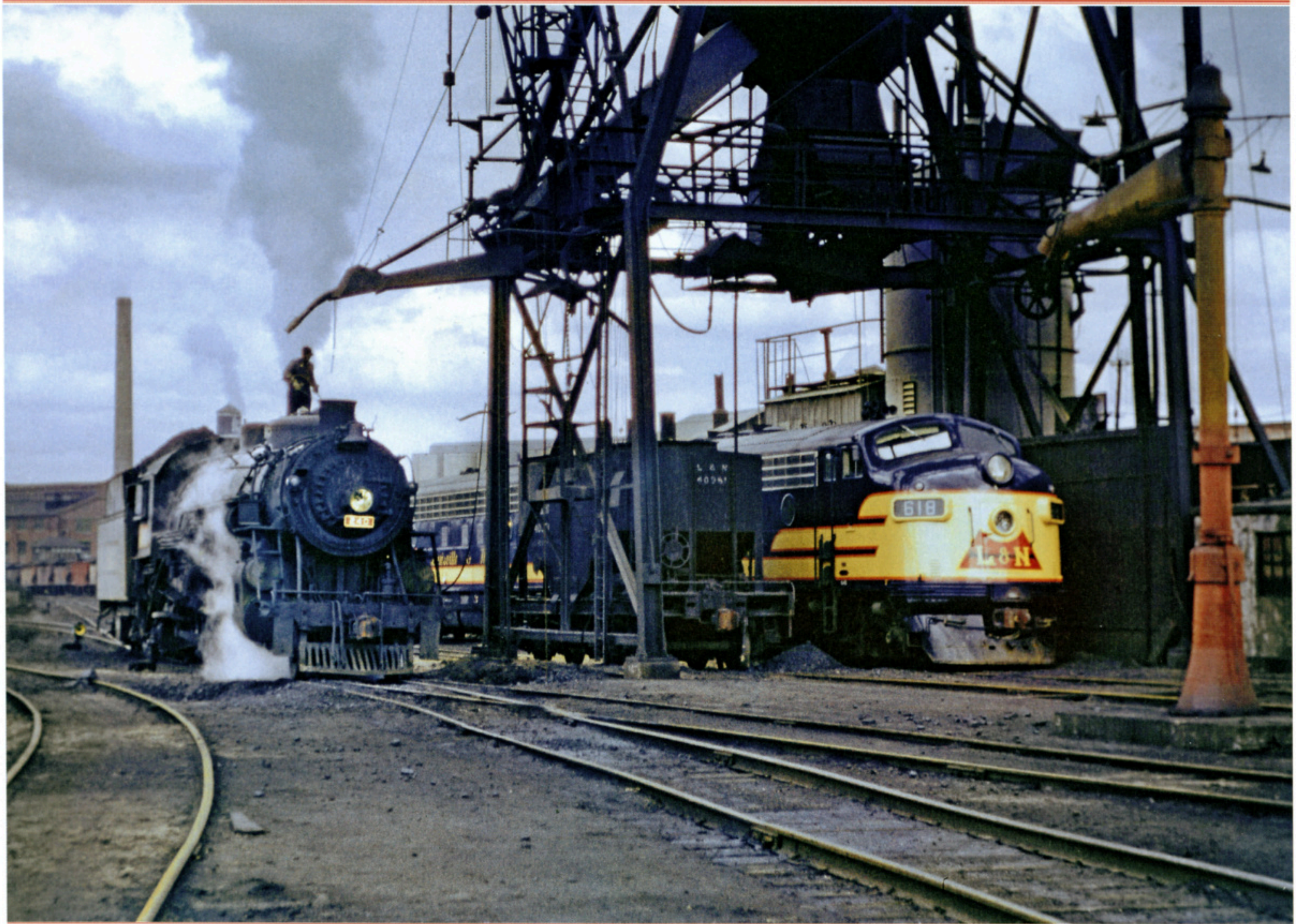
South Louisville's coaling and sanding facility plays host to the old and the new in this scene from 1951. K-5 Pacific 240 is being serviced before heading back to Union Station to handle a secondary passenger train. At the time of this photo, the 240 was assigned to the Cincinnati Division while FP7A 618 and her mates normally worked the Louisville Division. — Jack Fravert photo
