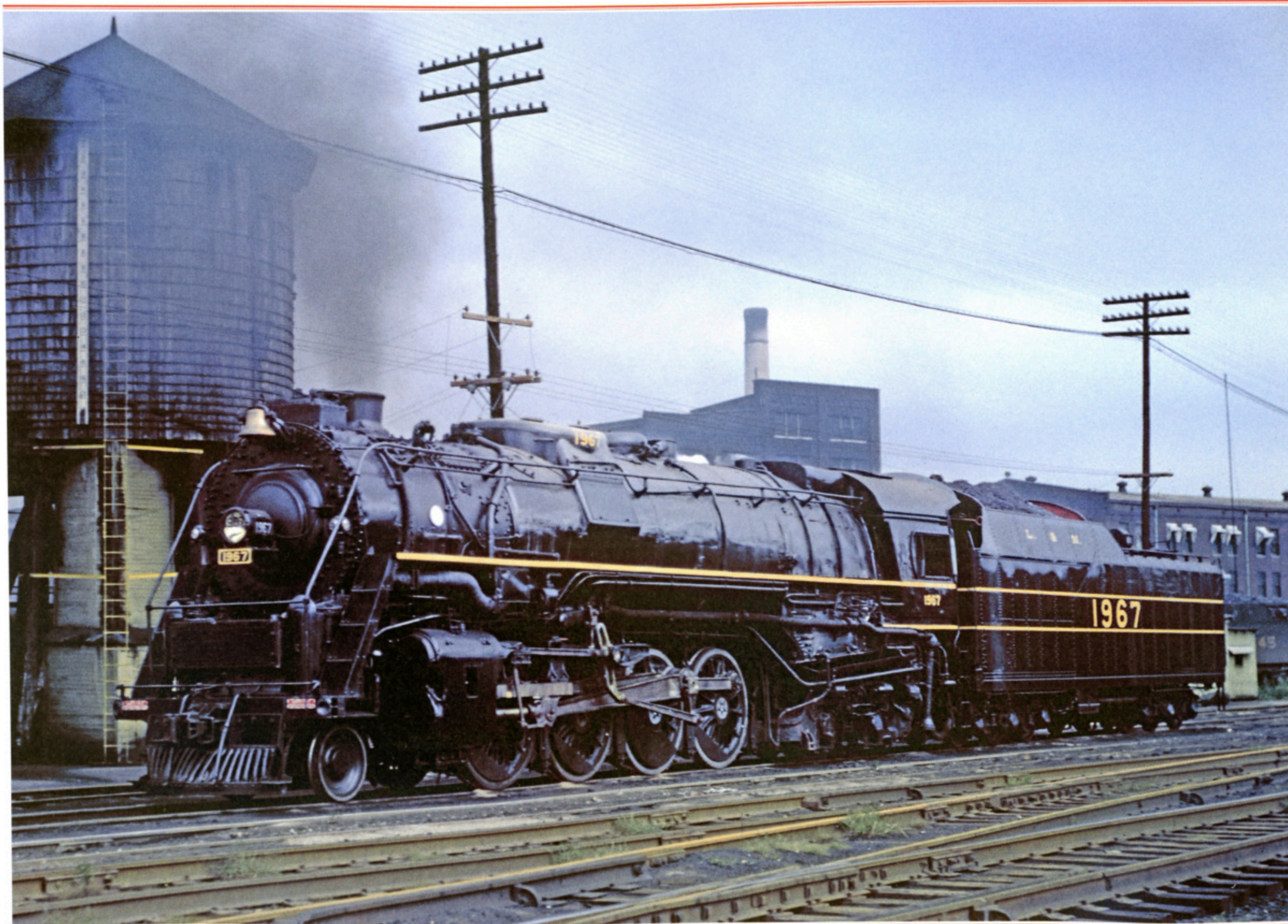
Just out of South Louisville shops after a Class 3 heavy rebuild in 1950, Baldwin-built M-1 1967 looks as good as when it first rolled out of the plant at Eddystone, Pennsylvania in 1944. The shine will be gone soon, however, after the engine rejoins its 41 sisters in heavy freight service on the "KY" Subdivision of the Cincinnati Division, the Eastern Kentucky Division, and the Cumberland Valley Division. —Jack Fravert photo
