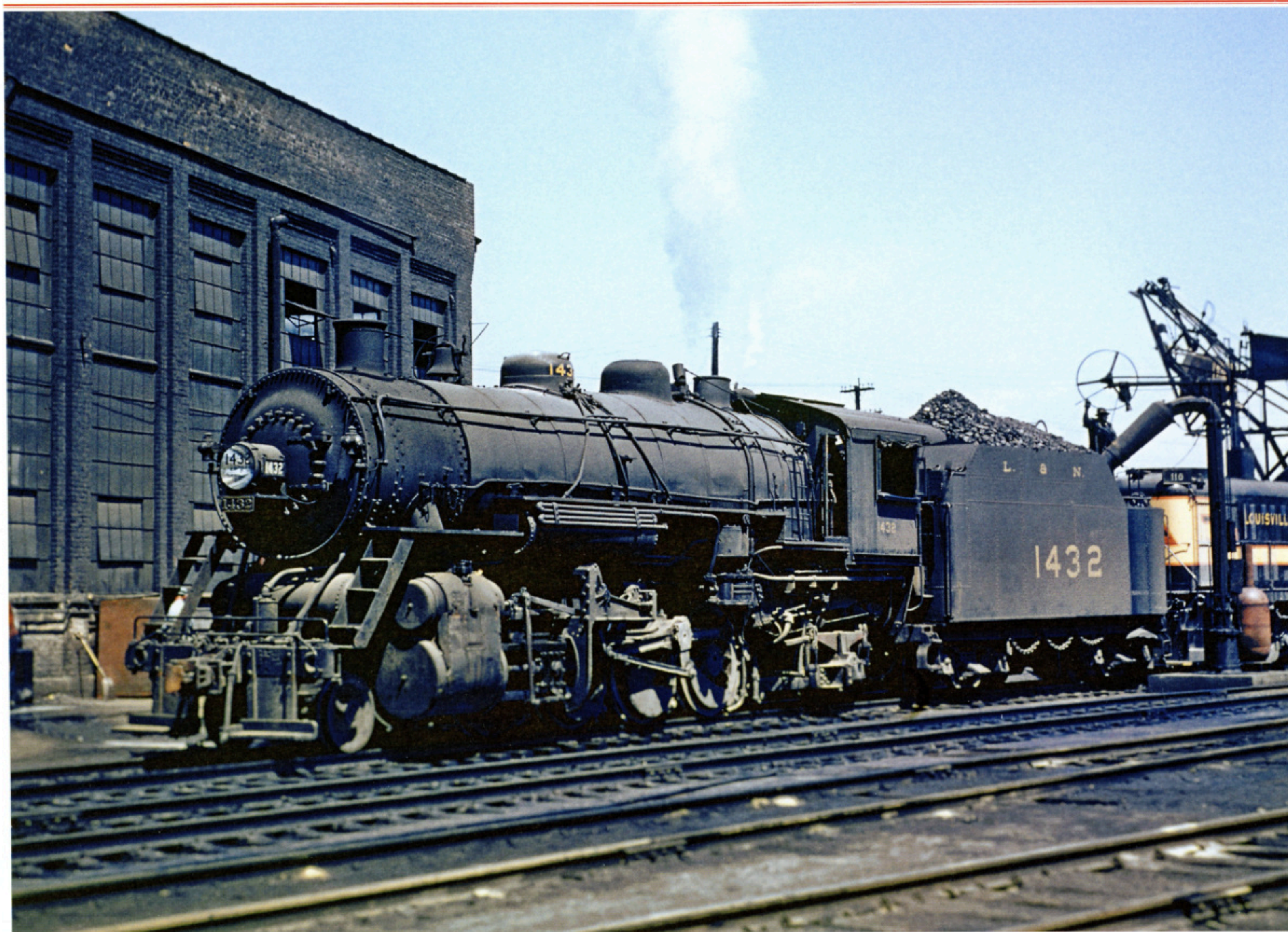
L&N Homebuilt (at South Louisville) J-1A Mike 1432 is shown beside the 26-stall roundhouse at DeCoursey, Kentucky in 1953. The L&N employed engines of this class in hump and interchange work in the Cincinnati area. The J-1As weren't fancy engines at all, but they could crank out 61,000 pounds of tractive effort — just 2,000 less than the heavy USRA-design J-4s featured on main line tonnage freights. — Jack Fravert photo
