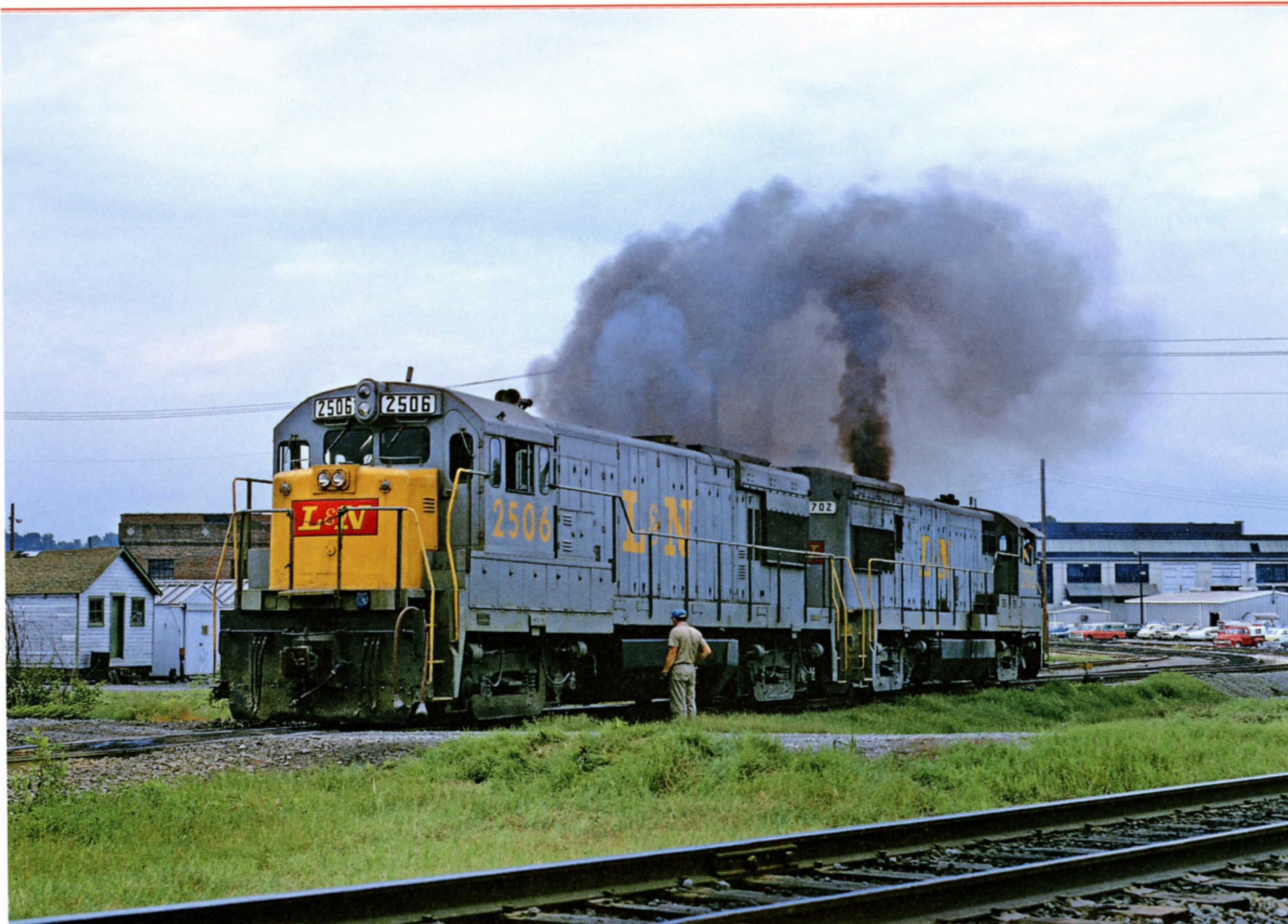
A hostler is backing a pair of GE four-motor units before heading forward into the fueling and sanding gantry facility at Corbin, Kentucky on June 28, 1974. The 2506 is a U30B while the 2702 is a U23B first constructed as Monon 603. The plume of smoke from the 2702 is a tell-tale sign of a bad turbo. —Ron Flanary photo
