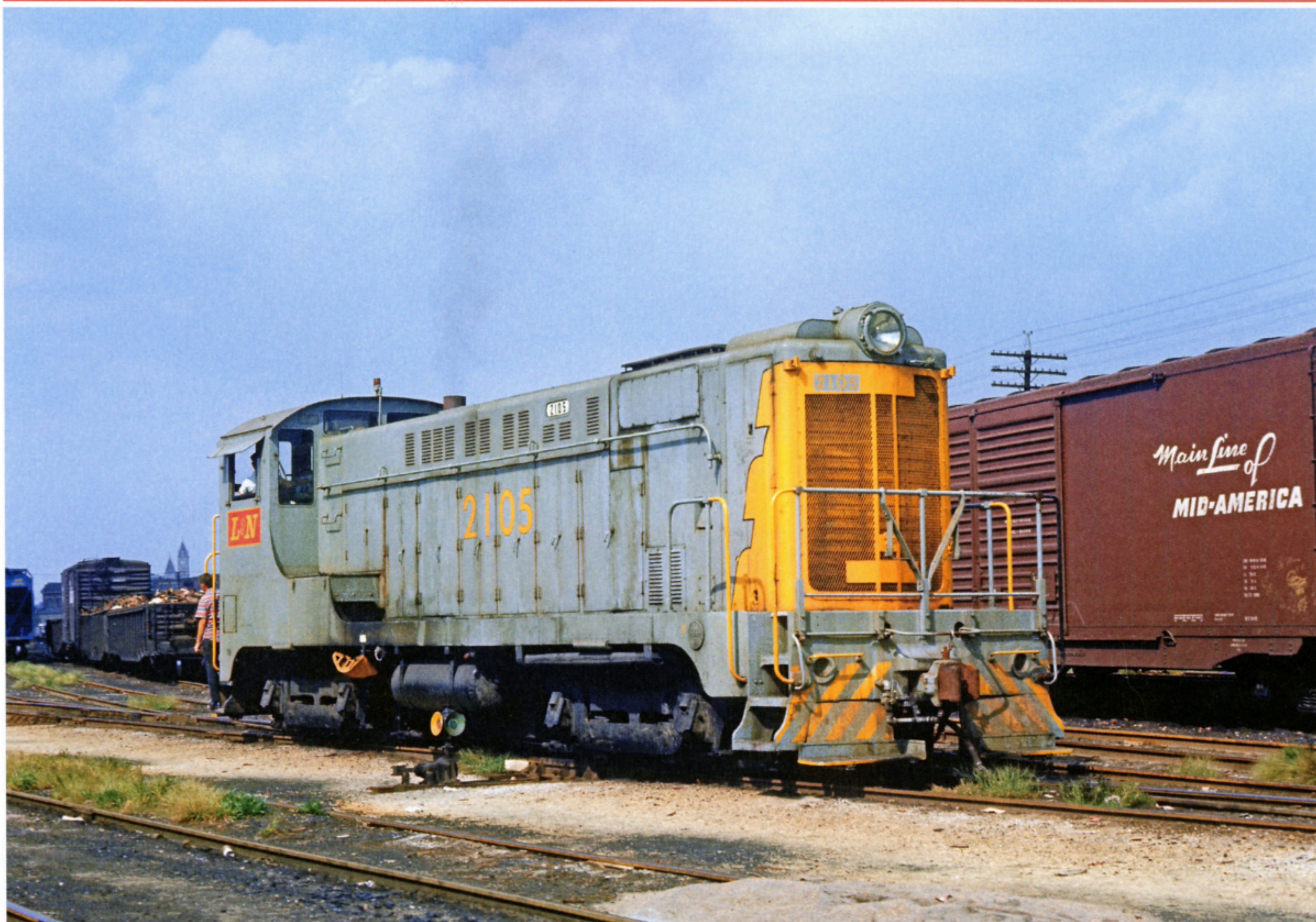
L&N Although classed by the L&N as an S-85, Baldwin switcher 2105 is a model VO 1000. The veteran unit, built in 1943, is shown working Oak Street yard in Louisville, just south of Union Station (which can be seen in the background) in September 1965. The 2105 was built as the 2205, but renumbered just a couple of months before this scene. She was retired two years later. —Jim Boyd photo
