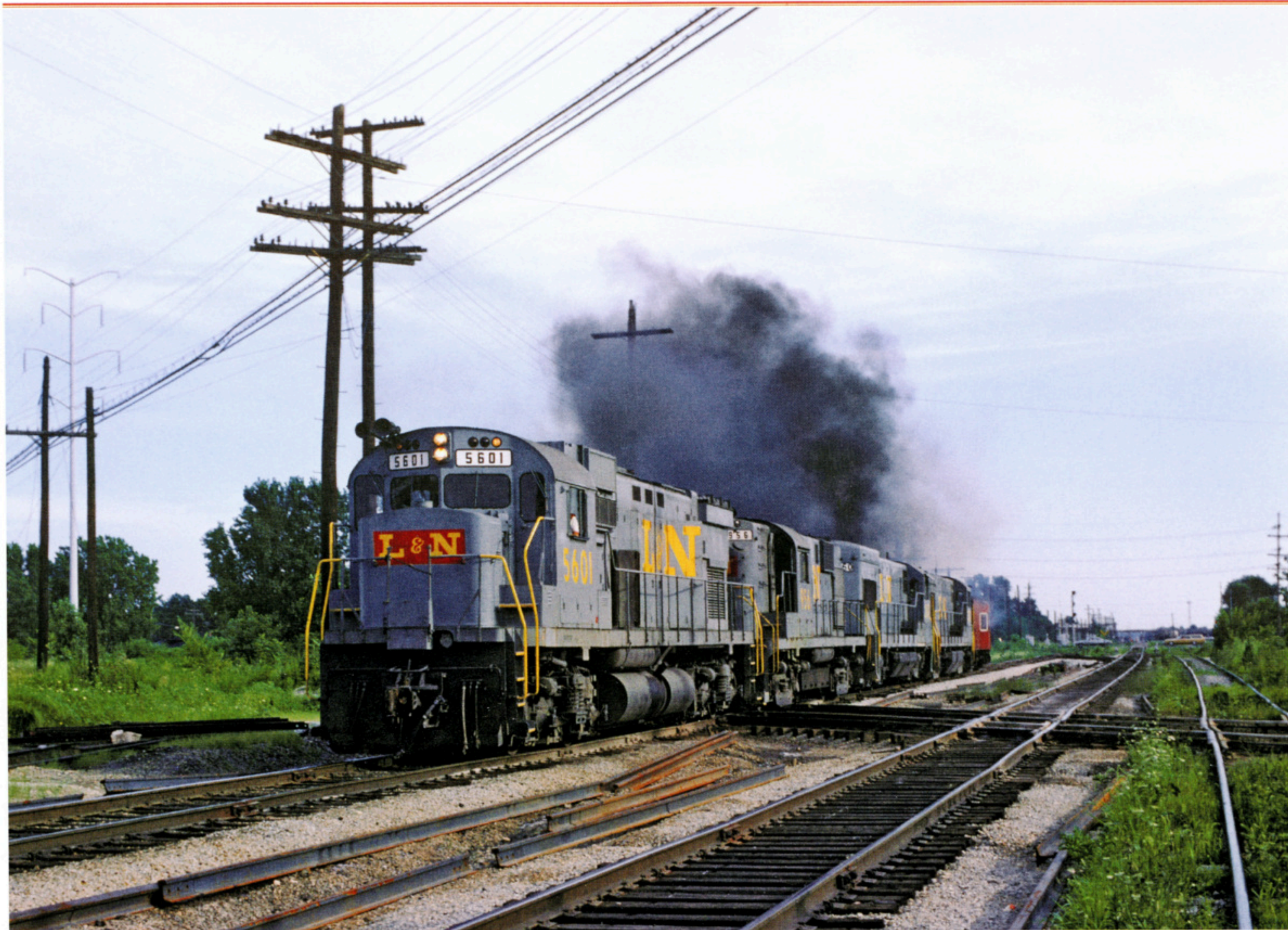
Two of the more rare units of L&N's diesel roster front a northbound extra "cab hop" at Dolton, Illinois in August 1977. Lead unit 5601 is a rare Alco C430 with high-adhesion trucks. The unit was built in 1967 as Alco demonstrator 430-2, one of three such engines. The trio was acquired by Seaboard Coast Line and eventually wound up in L&N ownership in 1976. The second unit is an Alco RS11 built in 1960 for the Seaboard Air Line and also coming into L&N ownership in 1976. Alcos were notorious for making "turbo lag" smoke if accelerated quickly, but in this photo, the culprit appears to be a GE U23B, third unit back. —Richard M. Panek photo
