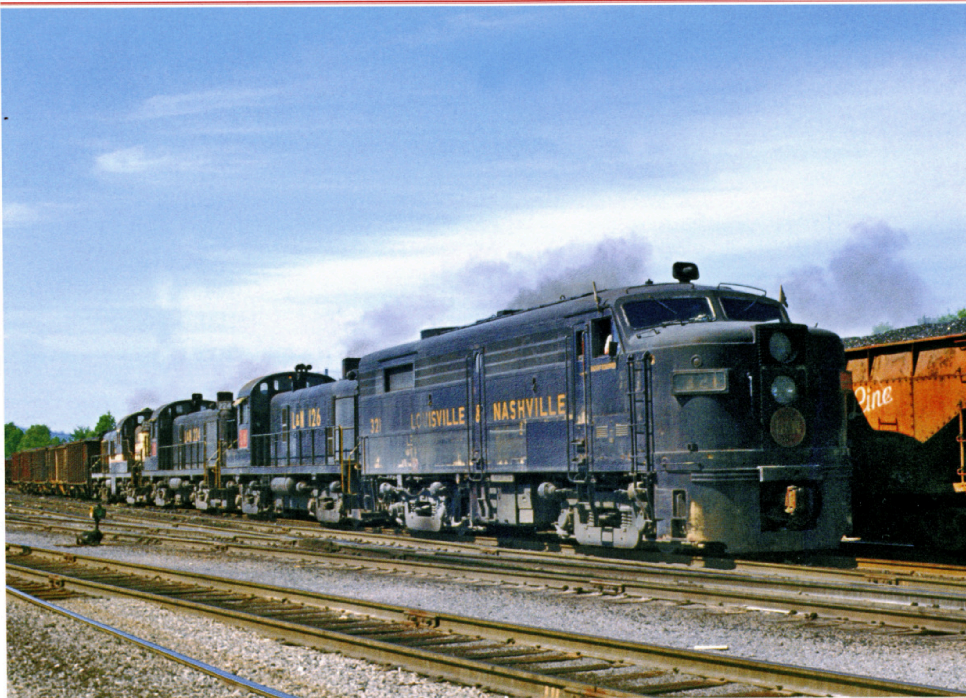
At Corbin, Kentucky's West Yard in September 1965, Alco FA-2 321 fronts RS-3s 126, 224 and 229 on a southbound extra freight for the Cumberland Valley Division. The 321 was the last cab unit Alco built for domestic service. After retirement for trade-in by the L&N in 1969 (to GE), the unit was one of six ex-L&N FA-2s purchased by commuter hauler Long Island Railroad for conversion to power cars. The former 321 operated many more years as LI 606. —David W. DeVault photo
