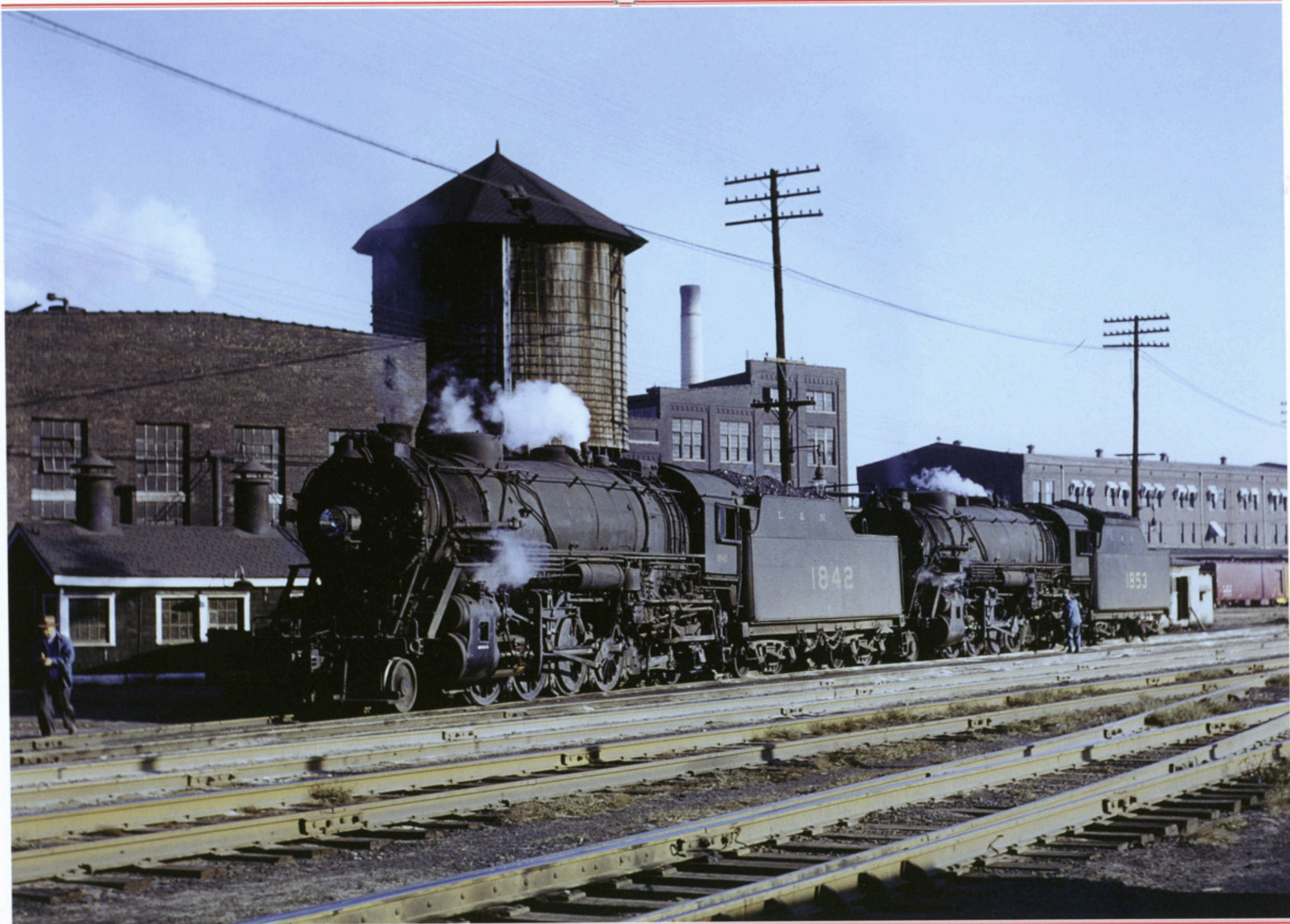
L&N Alco built 121 Class J Mikados for the L&N between 1923 and 1927, numbered 1770–1890. Two of the group, 1842 and 1853, are teamed up together at South Louisville in the early 1950s. Both of these 2-8-2s lasted until 1954; 1842 left the roster on September 15, and 1853 on April 23. The double-headed Mikes are called for an extra freight on the Short Line to DeCoursey. Tandem 2-8-2s were the norm on this tough “saw tooth” stretch of main line. — Jack Fravert photo
