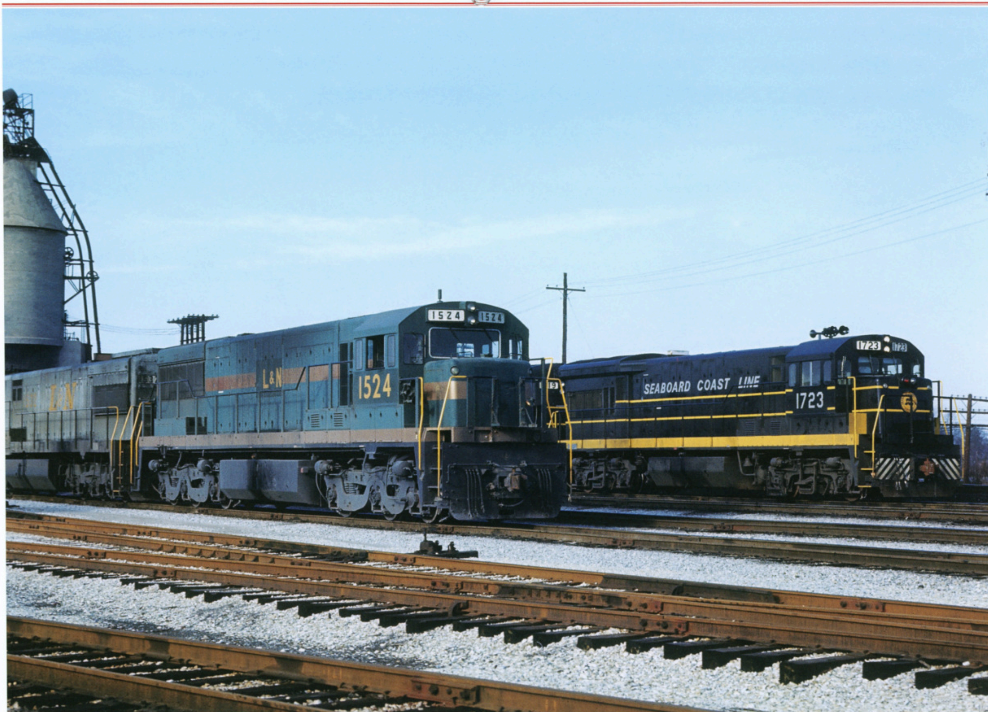
L&N This unusual photograph taken in Atlanta's Tilford Yard in January 1968 captures a wide variety of GE power, with each unit on a different kind of truck. Up close in front is ex-Oro Dam Constructors U25C 1524 riding on massive C-C trucks, one of eight the L&N bought, which is coupled to U28C 1532 riding on standard GE C-C trucks. In the background, SCL U33B 1723 rides on EMD's popular Blomberg B-B trucks. — Jim Boyd Photo
