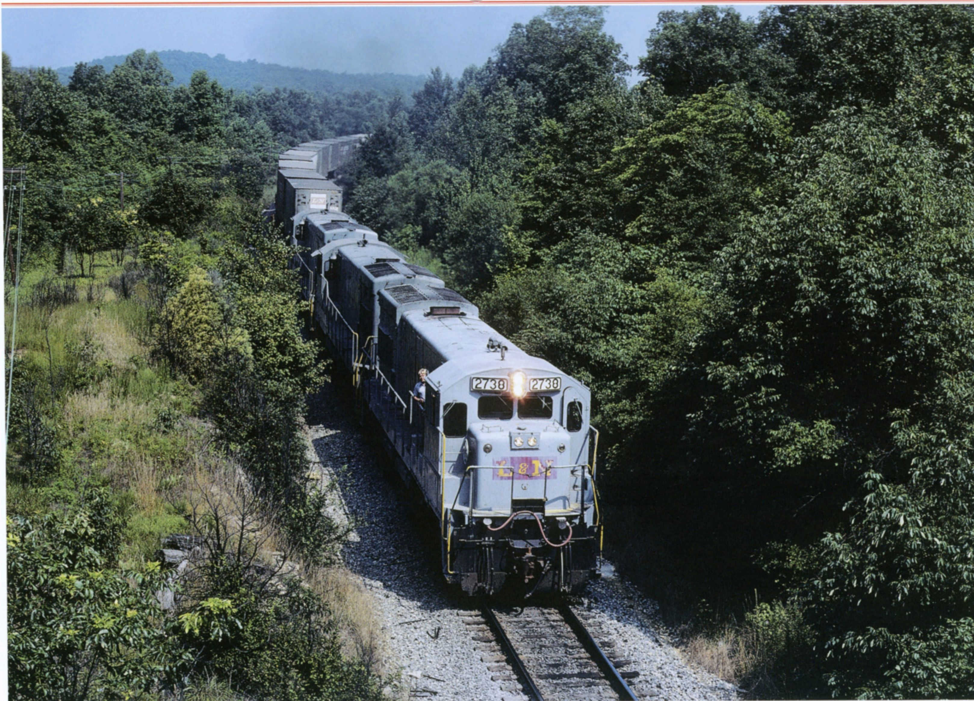
L&N A trio of U-Boats swings a southbound piggyback hotshot through Mannington, Kentucky, in August 1980. On the point is U23B 2730 wearing the solid gray scheme. The L&N long favored four-axle GE units for "Tote" trains ("Trailer On Train Express" — L&N's term for piggyback) such as this one. — Jerry Mart Photo
