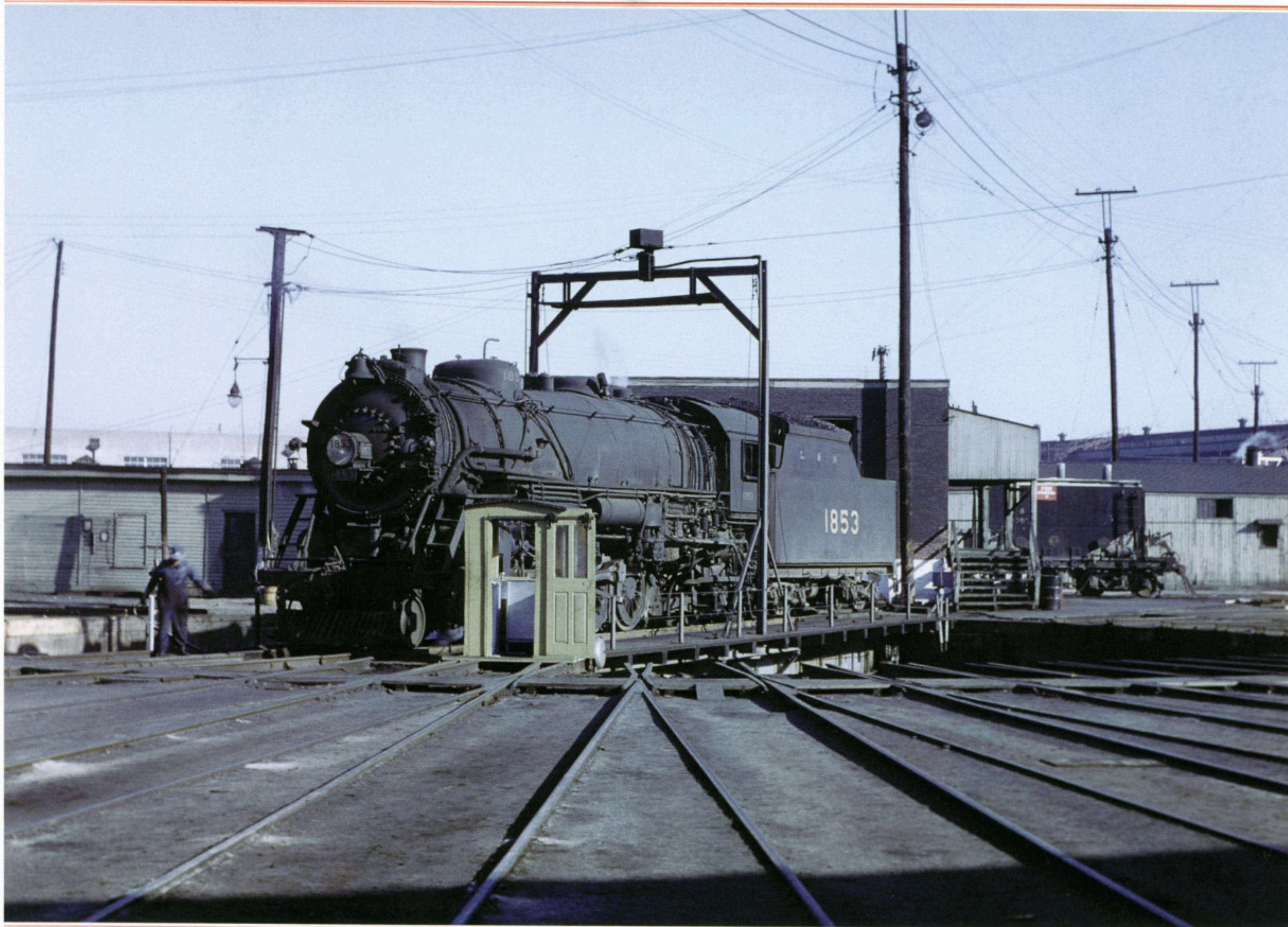
L&N The turntable in South Louisville gets some action as J-4 heavy USRA Mikado 2-8-2 1853 is turned in October 1951. The engine was retired on November 13, 1952, a matter of a few days after this photograph was taken. Ironically, the 85-foot South Louisville turntable was one of the smallest on the system for a main line terminal. Still, it could handle virtually anything the L&N had in steam except the M-1 2-8-4s. — Jack Fravert Photo
