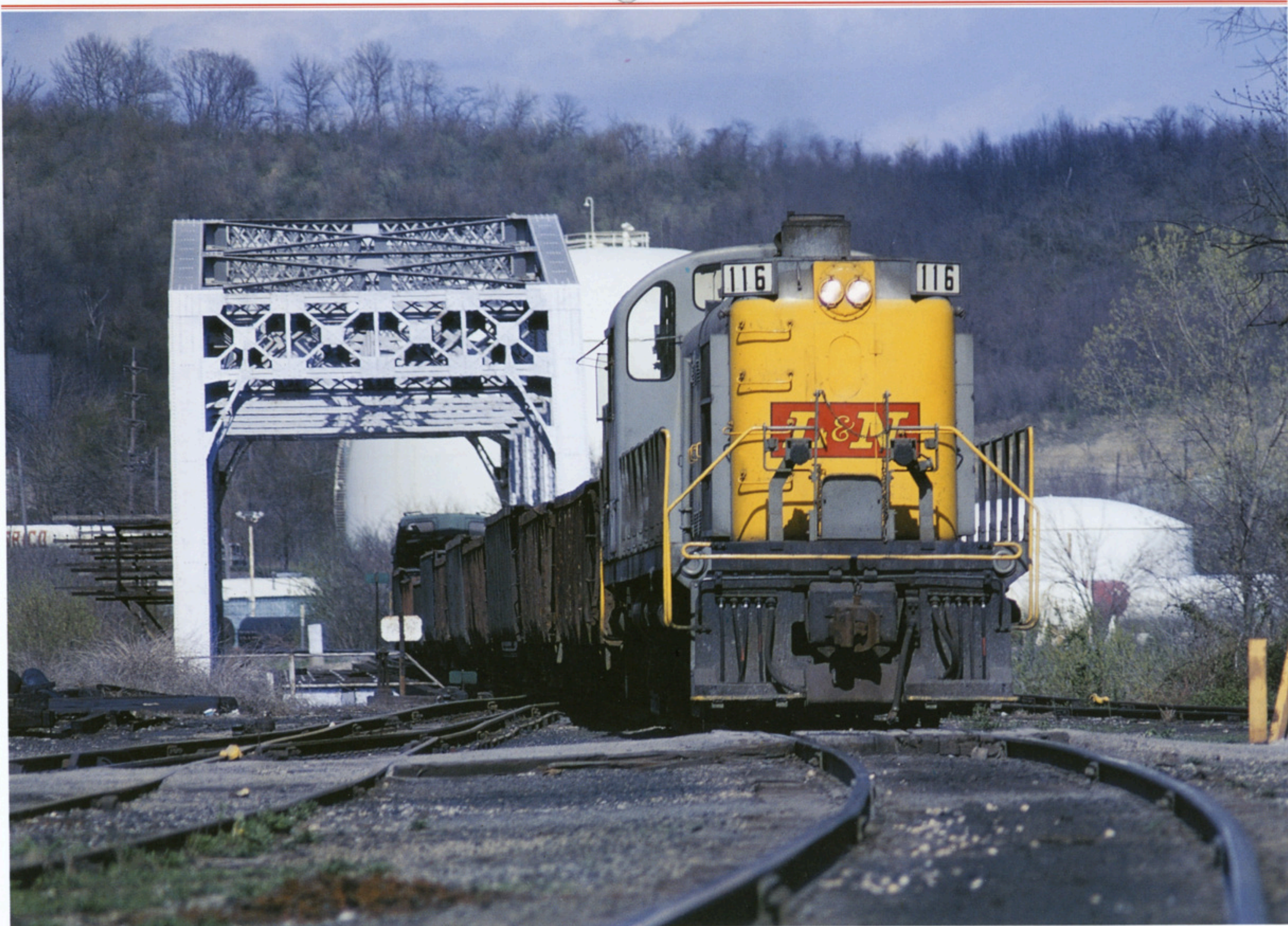
L&N This low-level view shows RS-3 116 ready for the next move at Latonia, Kentucky, on April 13, 1974. The short train is strung out across the Licking River bridge on the Wilder branch. The unit's Gryralight has been removed in a nod to greater efficiency and one less item to maintain. —Dave Oroszi photo
