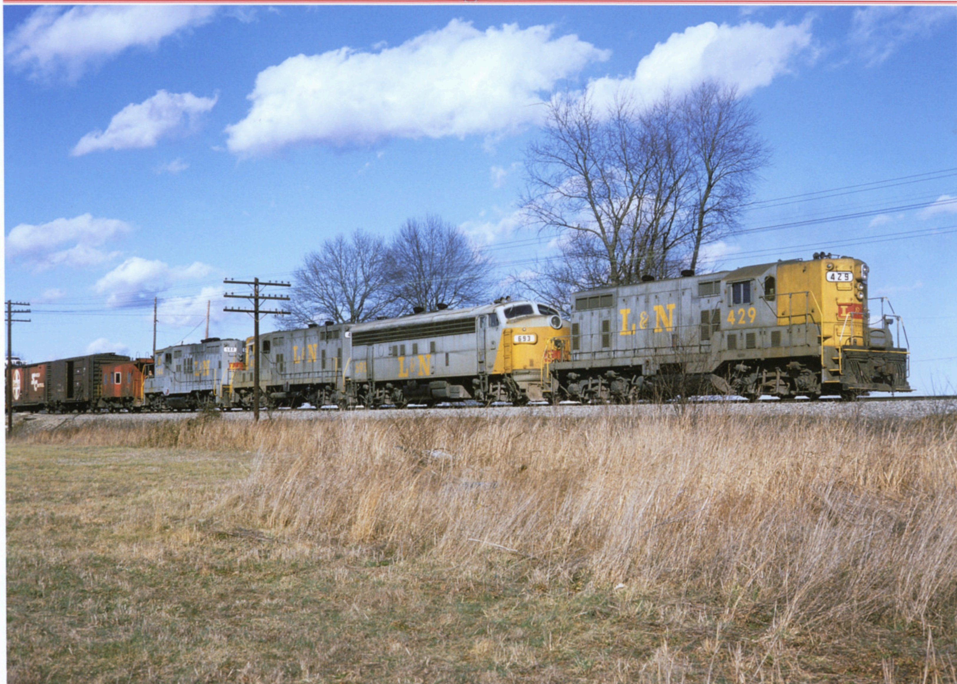
An all-EMD consist includes GP7 429 leads FP7A 693, a 450-series GP9, and GP9 544 northeast of Nashville at Galatin, Tennessee, in February 1975. The cab unit has but four months to operate before retirement. Now on its third road number, the 693 wears the final simplified version of the familiar gray and yellow L&N paint scheme. — J. Allen Hicks photo
