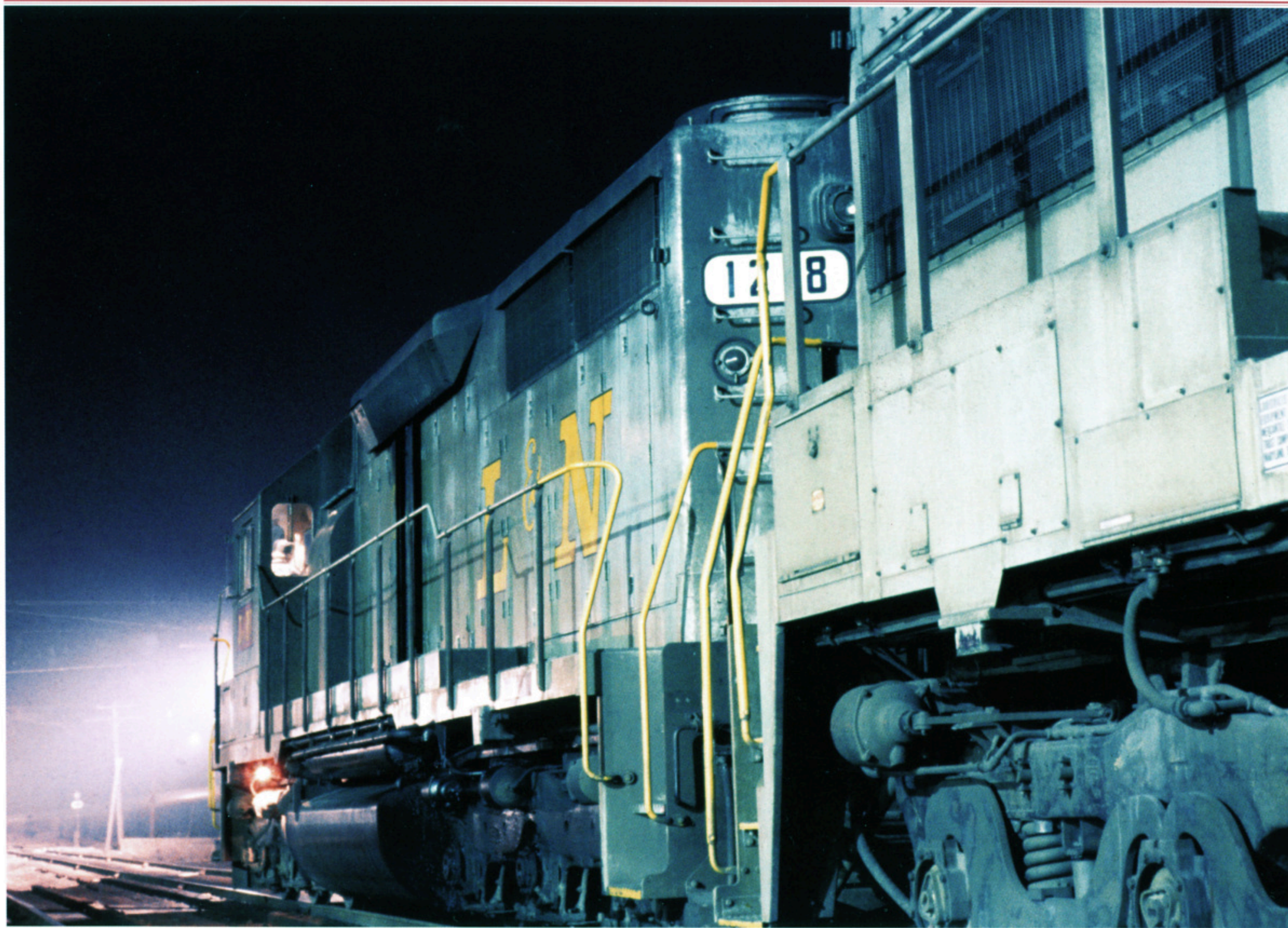
L&N Air compressors on SD35 1218 and U25C 1500 throb as the engineer rebuilds train line pressure after a set-off at Appalachia, Virginia, on February 10, 1968. Southbound freight 65 will soon throttle up for the final 10 mile climb to its eastern terminus at Norton, Virginia. — Ron Flanary Photo
