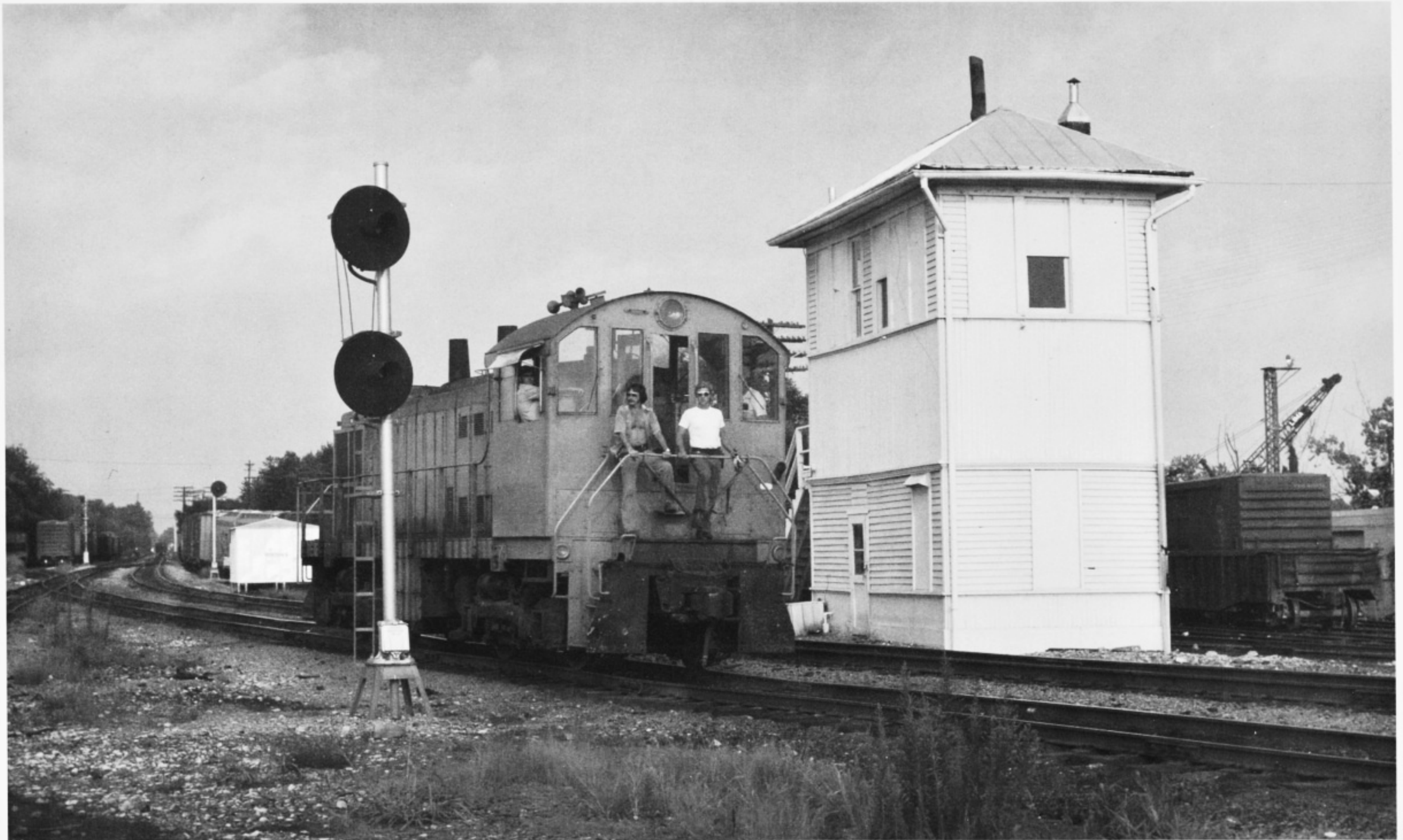
At MN Tower in East Louisville, the switchmen aboard L&N 39 are enjoying the breeze as they roll southward through the junction. The 1946-built Alco switcher was one of several to have its original 660 horsepower prime mover and electrical equipment replaced by an EMD 1200 horsepower diesel from a retired E-unit. The unique unit was photographed on April 18, 1981. (Dave Oroszi Photo)
