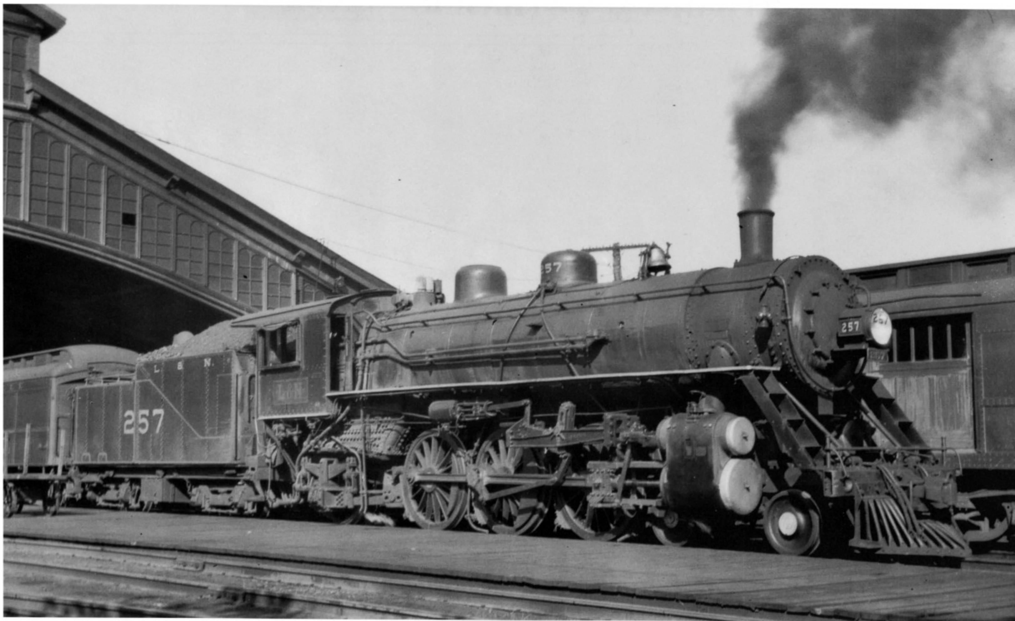
Coal smoke wafts from the tall stack of K4b Pacific 257 in front of the train shed at Montgomery during the mid-'30s. Although the light Pacific has been modernized with a power reverse, she's still hand-fired. The limited-clearance boiler tube pilot (which would not allow such engines to be coupled front-to-front) has not yet been replaced by a more practical stubby version. (Gary D. Rolih Collection)
