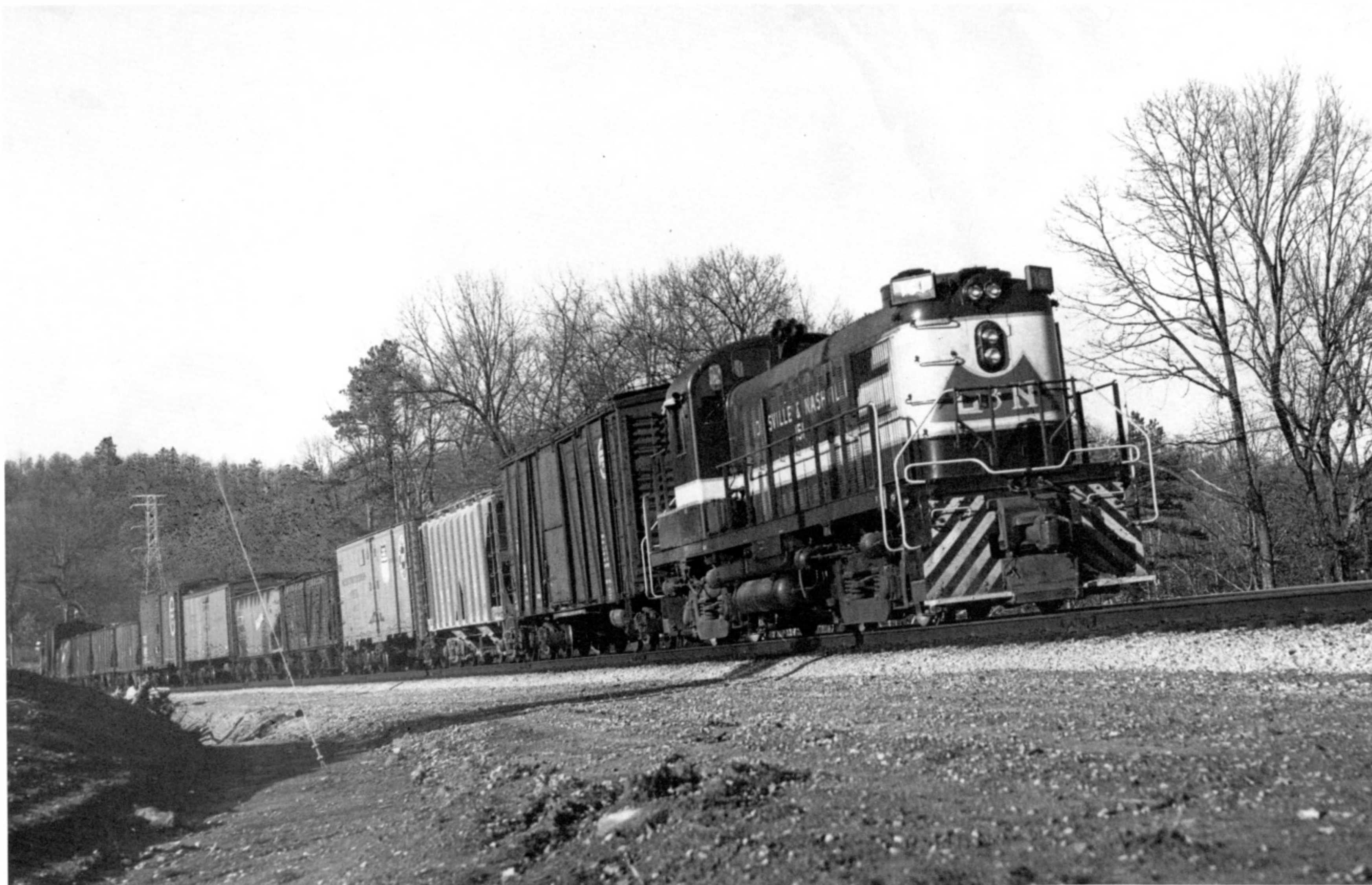
One of five (of 107 total) L&N RS3s with both a steam generator and Automatic Train Control (ATC), no. 151 handles a K&A Division local between Atlanta and Marietta, Georgia in 1953. As delivered, the 151 had no m.u. ("multiple unit") connections. (Dick Sharpless Photo)
