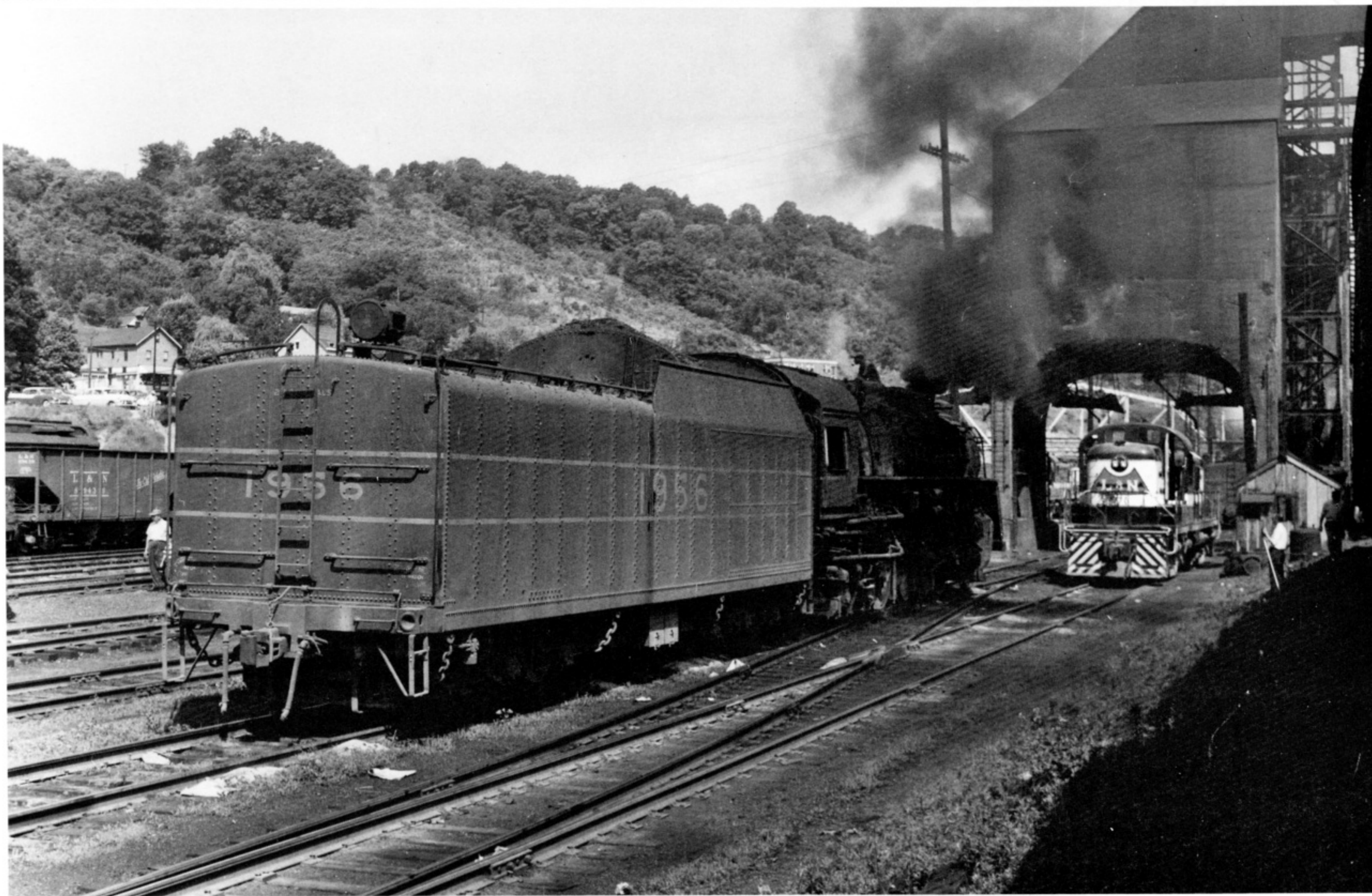
On June 24, 1956, railfans on the Cincinnati-Ravenna roundtrip excursion (behind M-1 1962) take in the sights at the DeCoursey roundhouse while the train makes a brief stop there. M-1 1956 is being serviced, and an RS3 is on the right. Note the "Emma's" back-up light—not original equipment. The coal pusher—a high maintenance item—has also been removed. (Jerry Taylor Photo/Ron Flanary Collection)
