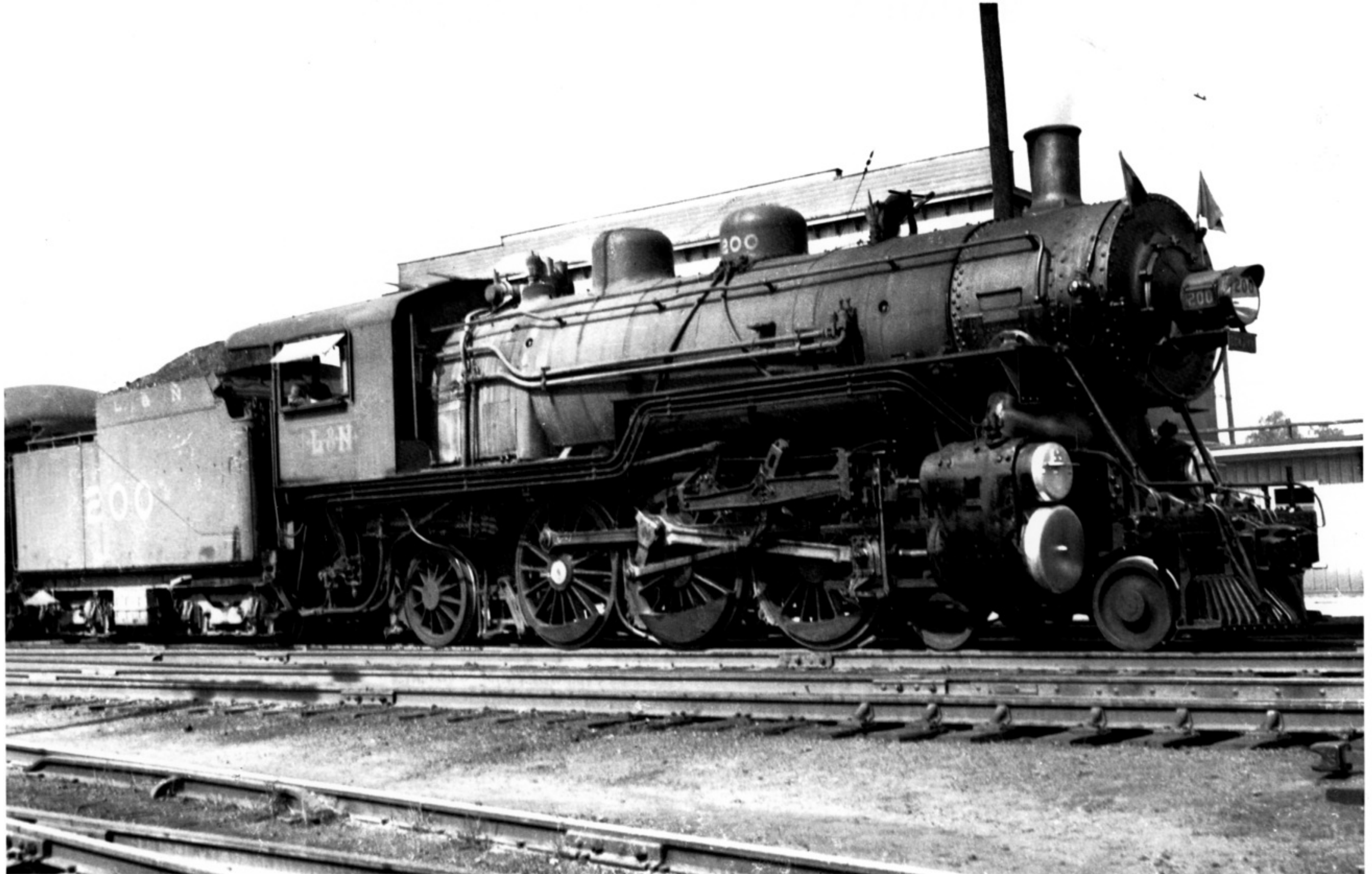
The engineer of K-3 Pacific no. 200 (built by South Louisville Shops in 1912) has the Johnson Bar "in the corner" for a fast getaway. This 1939 scene at Boyles, Alabama also reveals an indication of good things to follow: two green flags above the headlight tell us a following section will be coming. (J.E. Jones photo / Frank E. Ardrey, Jr. collection)
