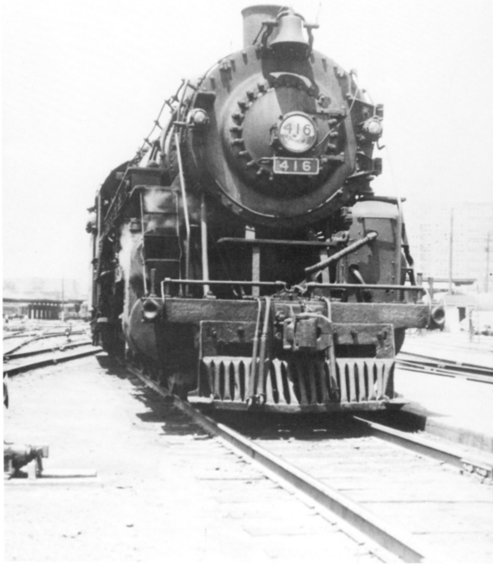
As the engineer looks back for a signal, L1 no. 416 backs into Louisville Union Station with train 7 for Nashville. From almost any angle, L&N's USRA-design "light" 4-8-2's were exceptionally good looking machines. (Charles B. Castner)
