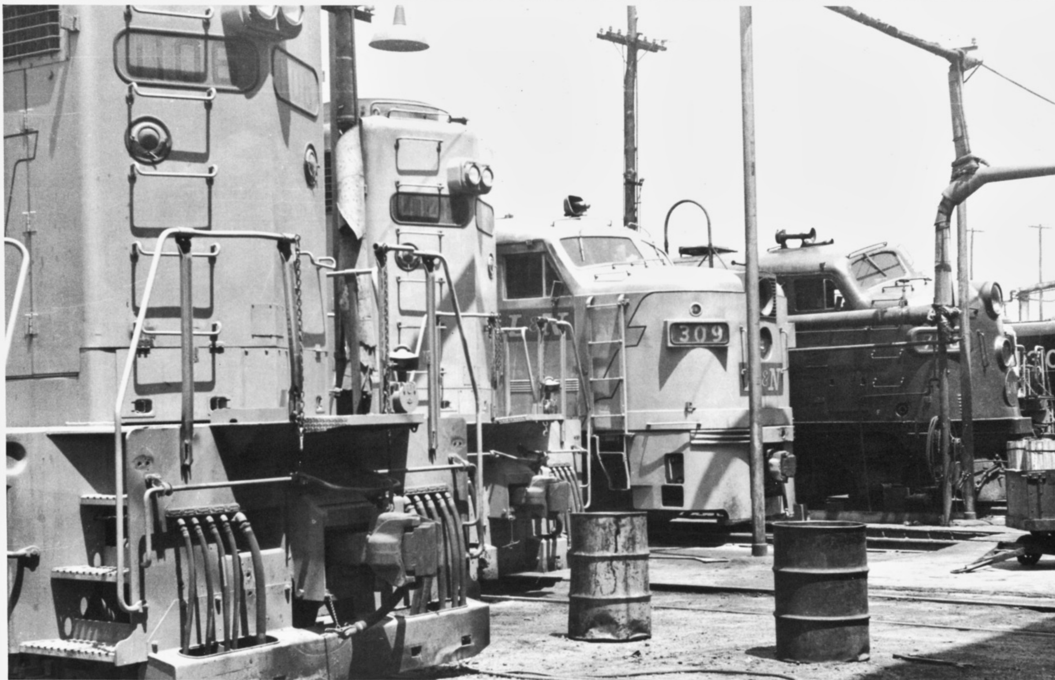
If pictures could talk, you would be hearing the wide open scream of a turbocharged EMD prime mover right now. In the days before such operations were moved into sound-insulated testing booths, GP35 no. 1106 (left) is undergoing a load test at South Louisville. This is Shop 17, the first system shop facility built for diesel repairs (designed for the E6 passenger units in the 40's). On this day in August 1965, the 1106 is joined by GP30 1046, FA2 309, E7 759, and a host of other unseen units. Shop 17 was usually full of L&N units of all types receiving running repairs. (Ron Flanary)
