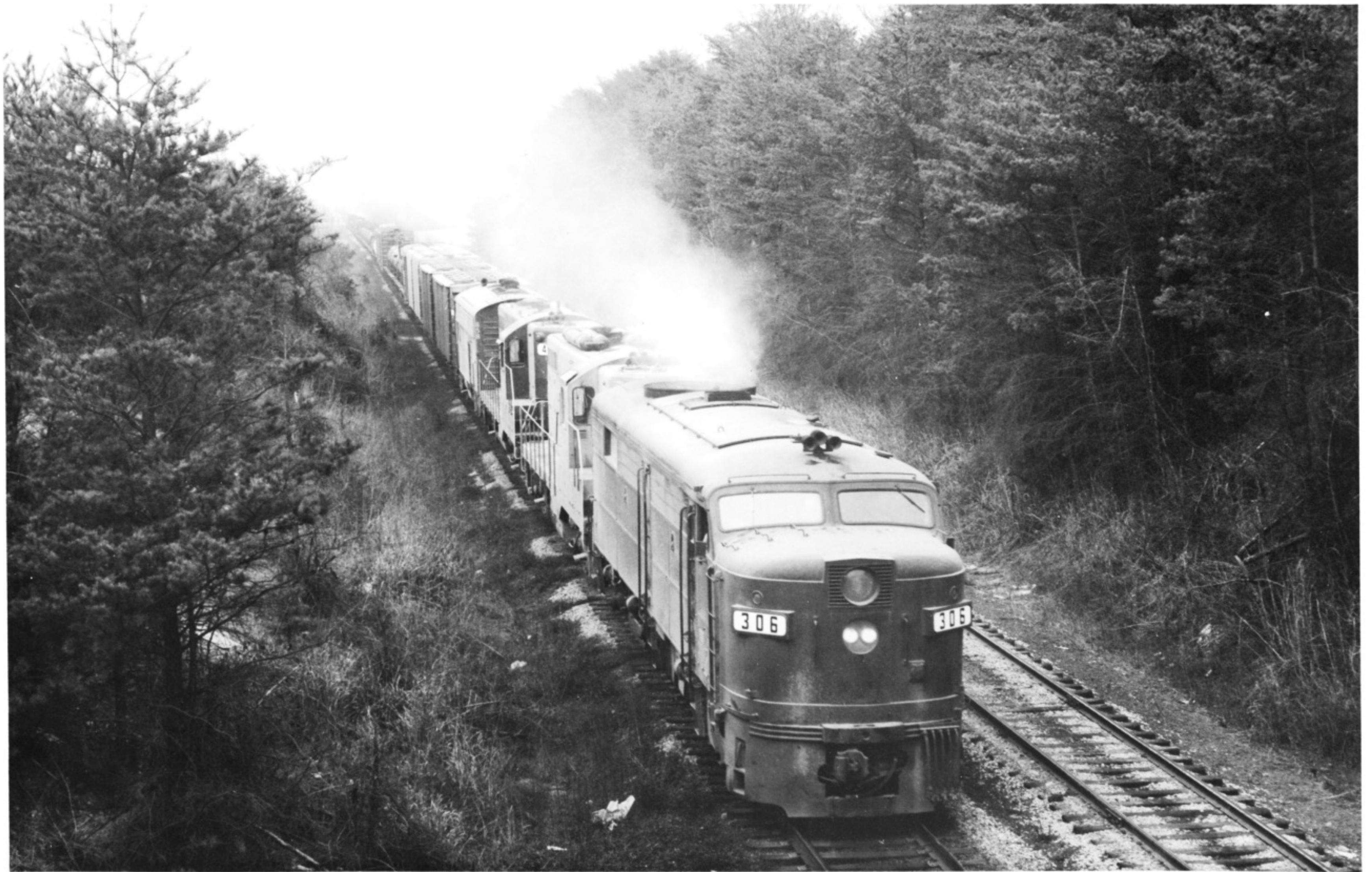
Standing on the U.S. 411 overpass just south of Etowah, Tennessee on March 16, 1966, the photographer captured this splendid action image of a southbound Knoxville & Atlanta Division fast freight behind units 306, 522, 414 and 858 (FA2/GP9/GP7/F7A). Alco FA2's had fronted K&A trains on this division for years, due primarily to many of them being equipped with Automatic Train Control, a requirement on the Etowah to Corbin segment of the division until mid-1964. With ATC deactivated two years previous though, the 306 is just another unit on the point of a freight. (Charles K. Marsh, Jr.)
