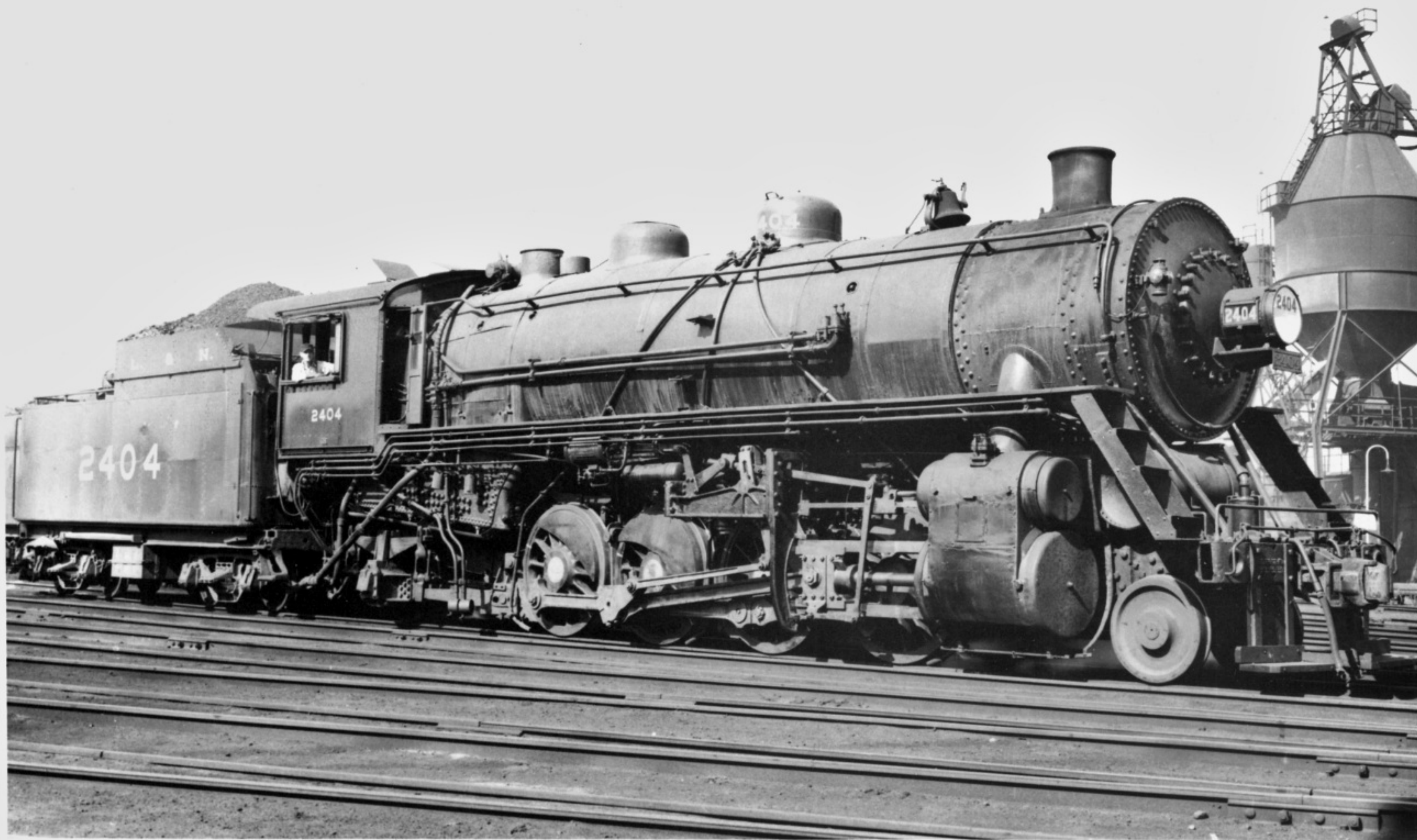
When L&N built its first 16 J1-class 2-8-2 Mikados in 1914 at its South Louisville Shops, it was decided to temporarily number them in the 2400- series until some equipment trusts could be retired. The beefy Mikes were pure drag freight era power, and spent most of their careers in the Eastern Kentucky coal fields and on transfer and hump duty in the Cincinnati area. For some reason the L&N never got around to renumbering the 2400's into the intended 1400-1416 slot, and they remained as the lonely occupants of the strange number series. The next order of J1's began with engine 1417. (R.E. Prince/F.E. Ardrey, Jr. Collection)
