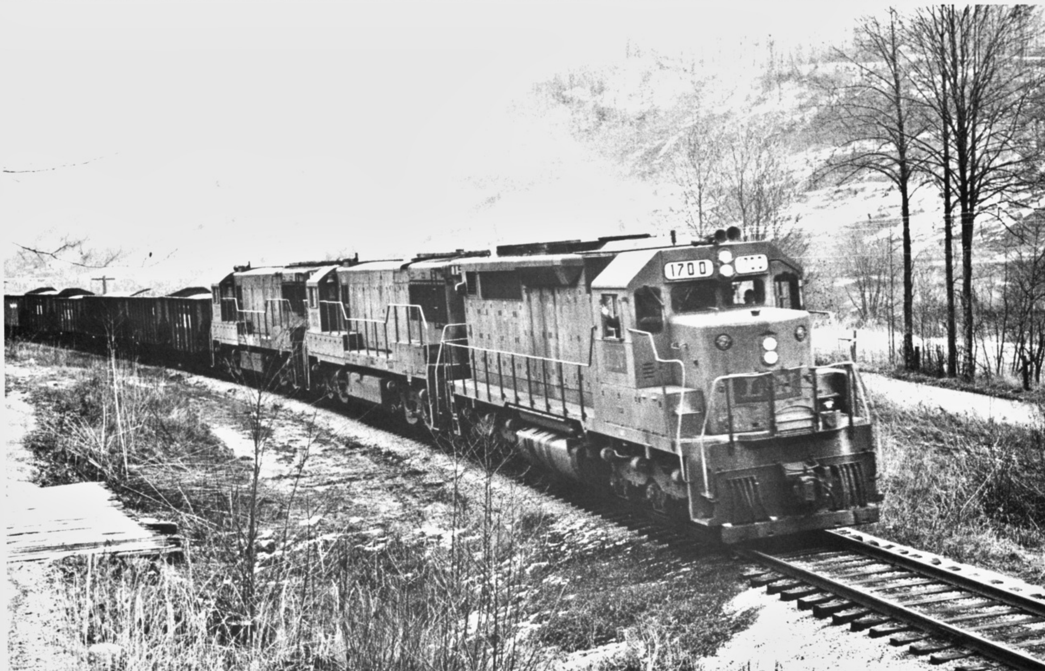
L&N's four SDP35's were strange creatures. Although they were designed to accommodate a steam generator, the units never got them. Consequently they never were placed into passenger service. The L&N did put the extra space in the rear of the long hood to good use to house radio control gear for the short-lived "RMU" (Remote Multiple Unit) operations in Eastern Kentucky. On February 2, 1968, "class" unit no. 1700 is just another six-axle freight motor as she works CV fast freight no. 864 near Olinger, Virginia. U25C units 1502 and 1513 trail the unique EMD. (Ron Flanary)
