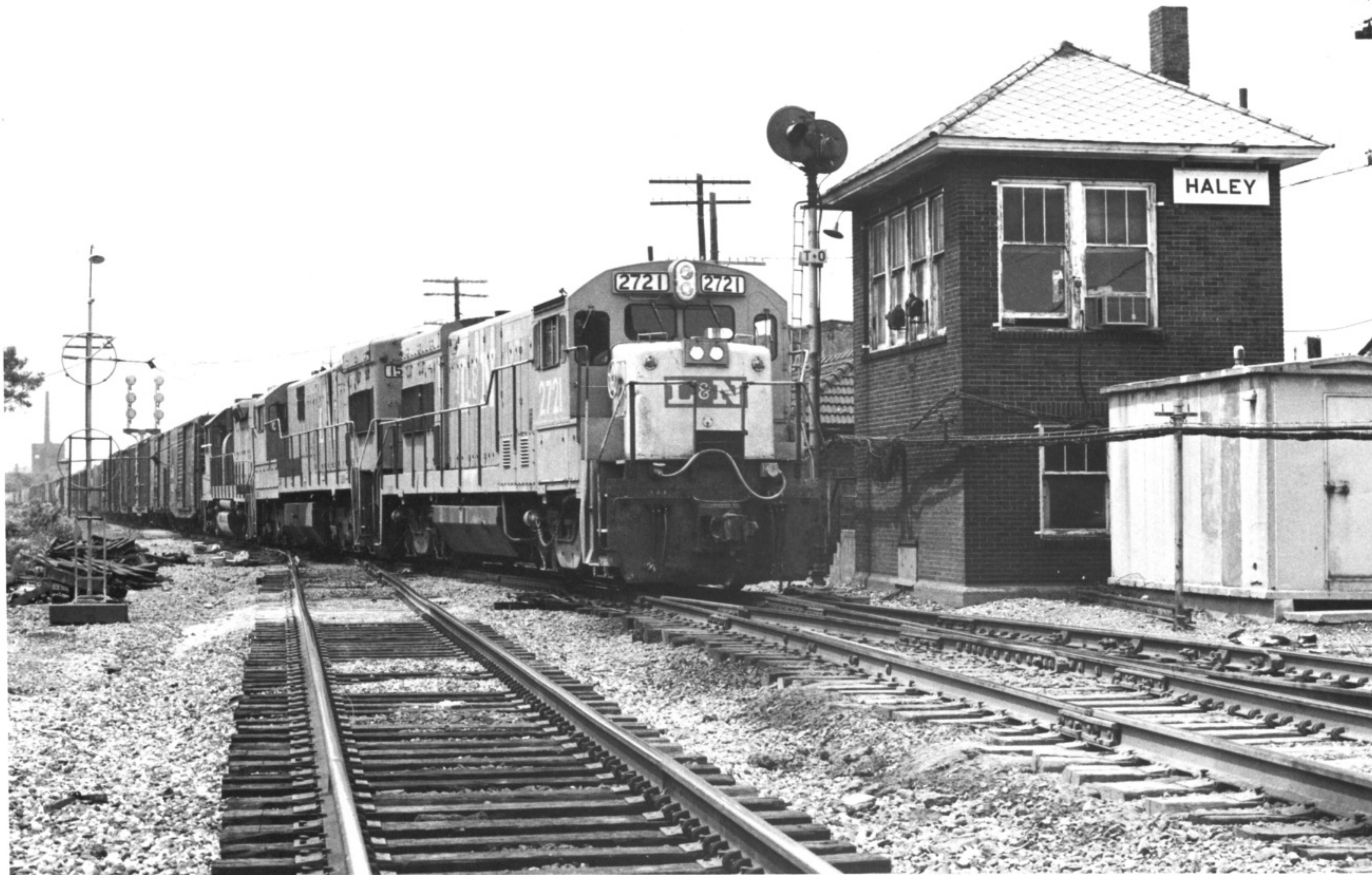
We're on ex-C&EI trackage at Haley Tower near Terre Haute, Indiana as northbound freight 718 hits the Conrail crossing in a cacophony of metal on metal. The double track is the former New York Central Indianapolis-St. Louis line. The Chicago-bound L&N freight is powered by 2721/1581 and 4087 (U23B/U30C/GP38-2). (Dave and Jill Oroszi)
