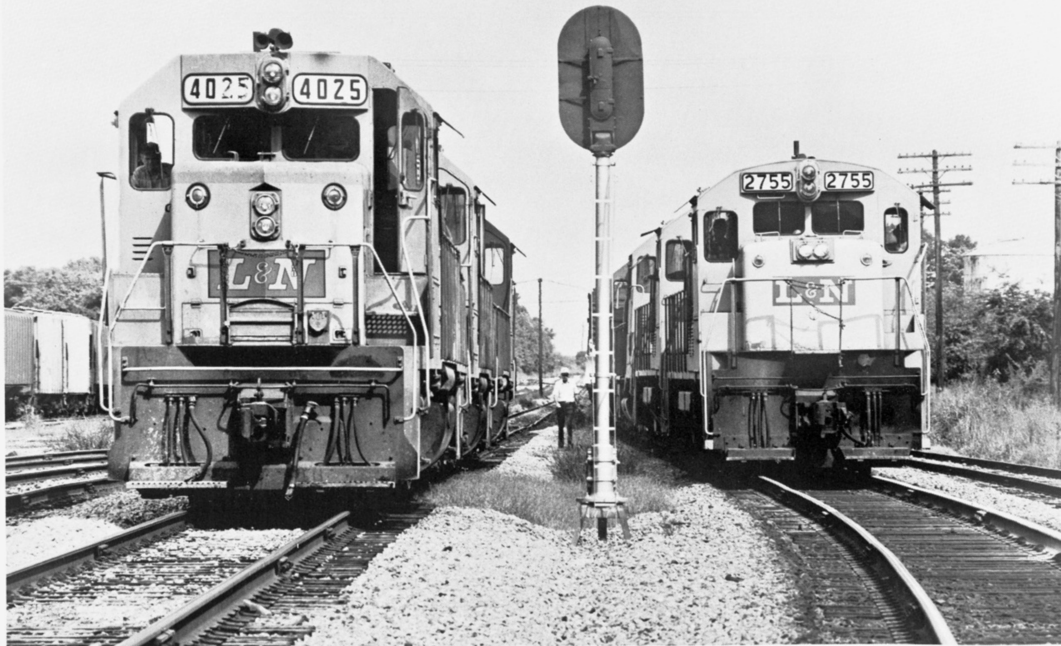
Cowan, Tennessee has been a pusher terminal since rails were first laid across Cumberland Mountain by the Nashville & Chattanooga Railroad in 1853. Carrying on the tradition established by Russian Decapods, dual 2-8-2s, and NC&StL's obscure 2-8-8-2s, three GP38s stand by to give a southbounder, led by U23B 2755, a push up to Cumberland Mountain Tunnel in August 1975. (J. Parker Lamb)
