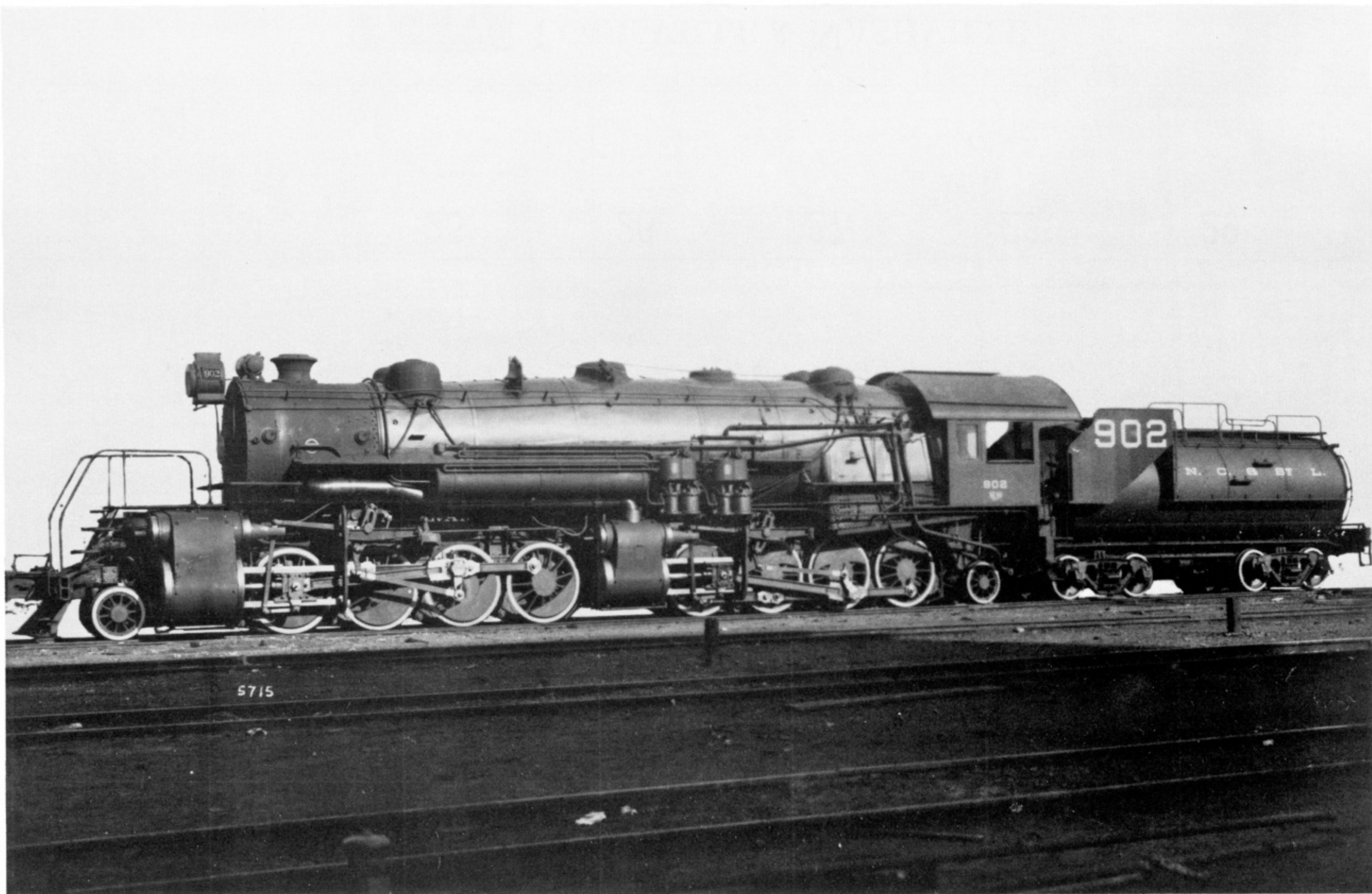
There were other M-1's in the L&N/NC&StL corporate family besides the "Big Emmas." In 1915 NC&StL purchased three burly compound 2-8-8-2's from Baldwin for helper service across Cumberland Mountain in Tennessee. The big engines, classed as M-1's by the NC, were assigned to Cowan, where they served with distinction until retirement in April, 1945. (L&N Photo)
