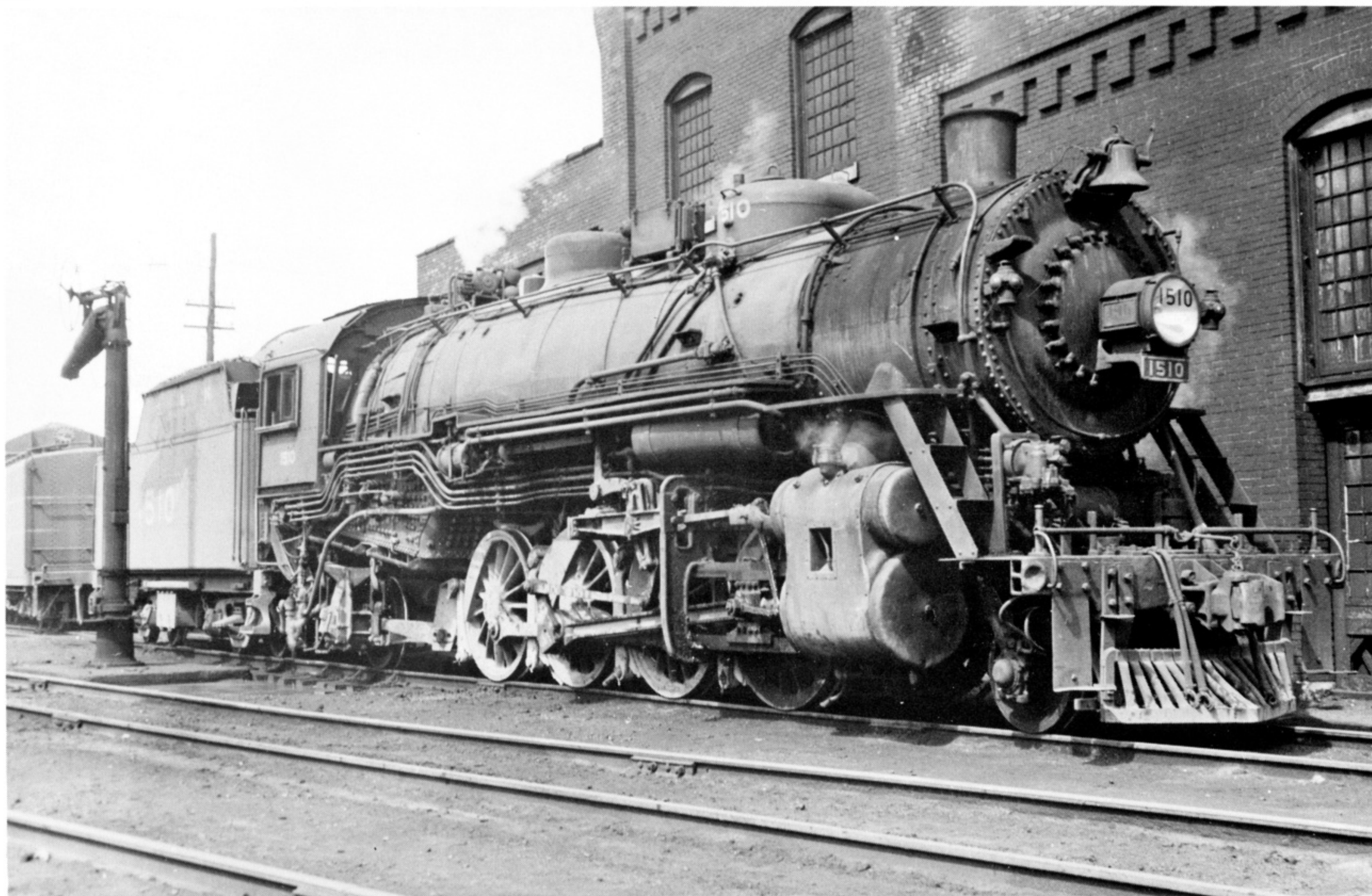
L&N's Knoxville & Atlanta Division was Automatic Train Control territory for many years (until it was finally retired in 1964). ATC - equipped J3 Mike 1510 shows off all her extra electrical appurtenances in this April 9, 1950 scene at Corbin, Kentucky. A Baldwin "Big Emma" waits behind, ready for another tonnage coal train bound for DeCoursey. (Railroad Avenue Enterprises)
