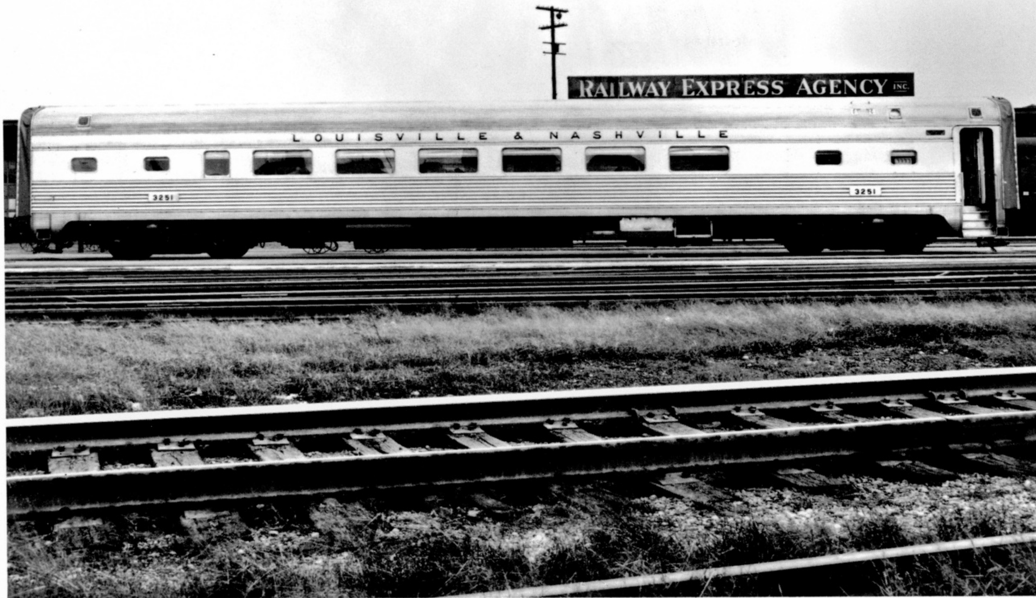
L&N coach 3251, built by the Budd Company in 1949, seated 52 passengers in deluxe comfort for service in the steamlined version of the Crescent . The stainless steel coach was eventually purchased by Amtrak and renumbered 6068. The Railway Express sign is not on the roof of the car but on a building behind in this scene shot in Louisville. (L&N)
