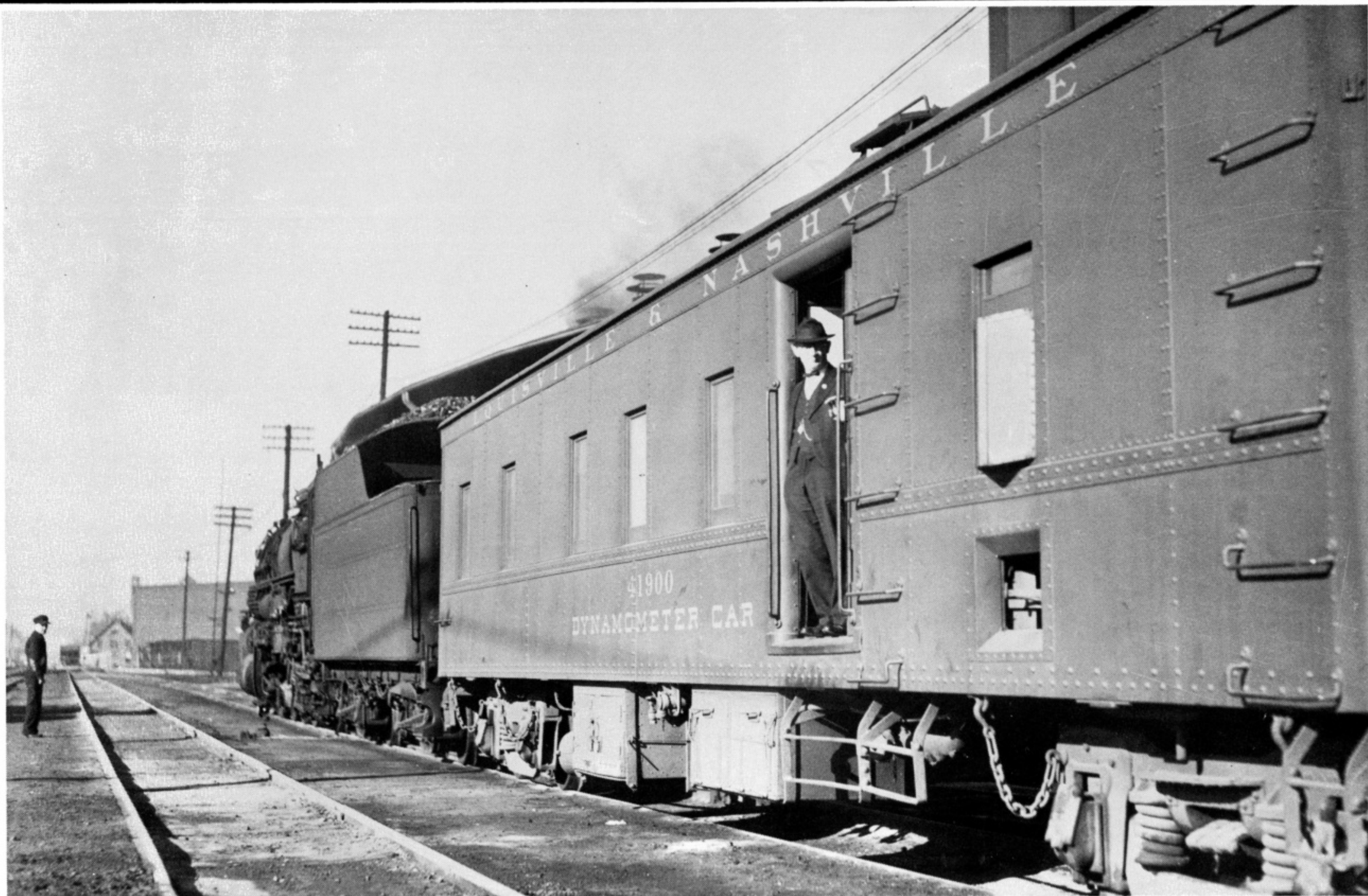
A few years before L&N began purchasing new road power in the early 40's, the home road arranged to purchase dynamometer car 41900 from the NC&StL to handle locomotive testing. This unique piece of equipment had been purchased by the NC in 1917 and numbered 90130. It's shown at the South Louisville roundhouse coupled behind what appears to be a J4 Mike. (L&N)
